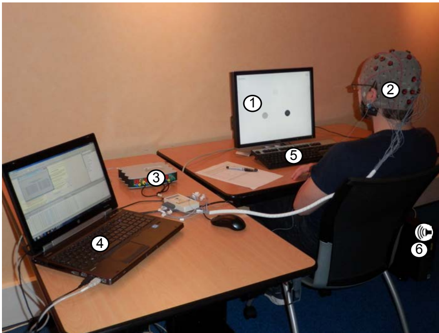
Figure 3.2: Experimental setup. 1: Visual display. 2: g-tec EEG headset. 3: EEG signal amplifier. 4: Laptop for EEG signal processing. 5: Keyboard. 6: Computer handling the stimulations and the instructions (either as displayed or audio text)
