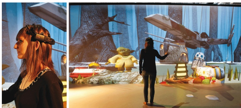
Figure 2.14: The Dagobah immersive setup, where the user has to focus to lift objects [Lécuyer et al., 2013]
