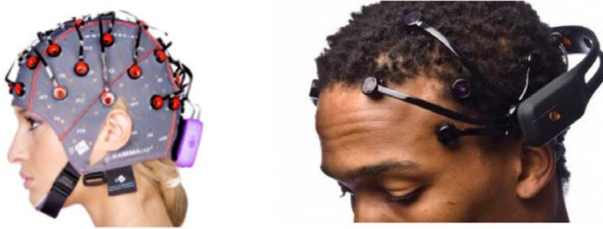
Figure 1.2: Left: g-tec EEG headset, with 32 g.LADYbird active electrodes. Right: Emotiv EPOC low-cost EEG Headset, using dry electrodes 4
