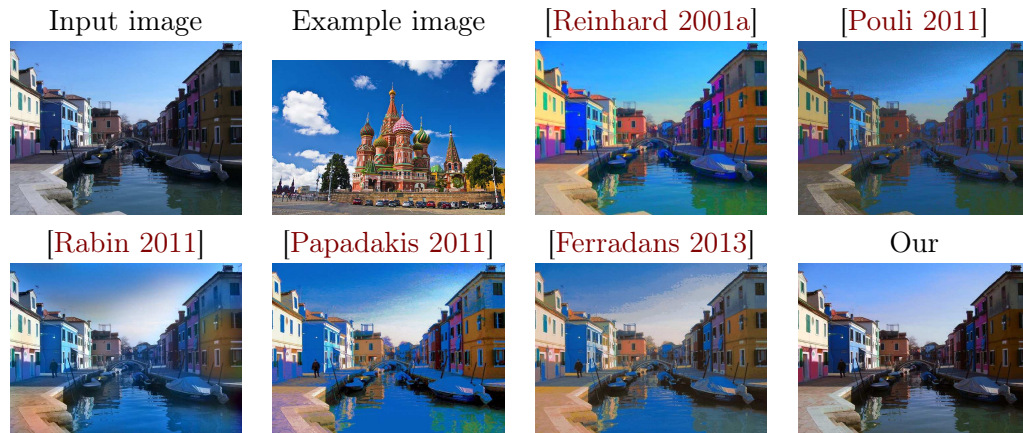
Figure 4.5: Results obtained by state-of-the-art color transfer techniques compared to our method for the Burano/moscow pair. While state-of-the-art techniques generate inconsistent color mapping (sky halo, incoherent color on the water), our method leads to a visually plausible and artifact-free result. Images are best viewed in color and on the electronic version.
