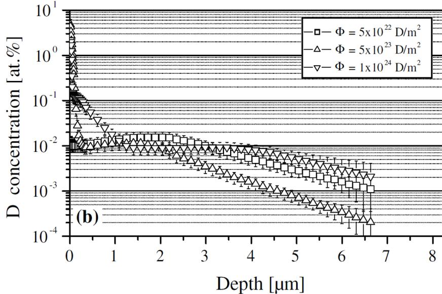
**Figure 2.9.** NRA depth profile of D in SCW irradiated with 200 eV/D ions with a flux of  $1.8 \times 10^{18} \text{ D} \cdot \text{m}^{-2} \cdot \text{s}^{-1}$  at 300 K. Figure taken from Alimov et al. [89].
