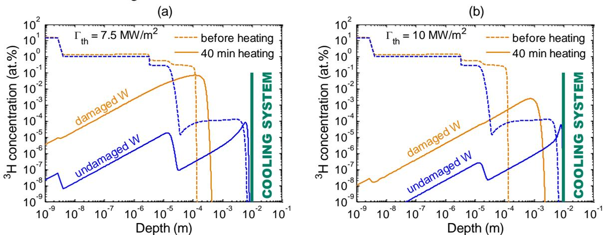
**Figure 5.10.** (a) Simulated  $^3\text{H}$  depth profile in damaged (orange) and undamaged (blue) W after 10 cycle and before the surface heating (dashed line) and after 40 min of heating (solid line) with a heating flux of  $7.5 \text{ MW/m}^2$ .
