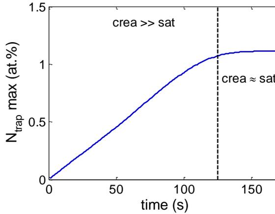
**Figure 4.7.** Evolution with time of the maximum trap concentration in the 10 nm zone during the implantation phase at 300 K. For this simulation, the incident flux is  $6 \times 10^{18} \text{ D} \cdot \text{m}^{-2} \cdot \text{s}^{-1}$  and the fluence is  $10^{21} \text{ D} \cdot \text{m}^{-2}$  (the implantation last 167 s).
