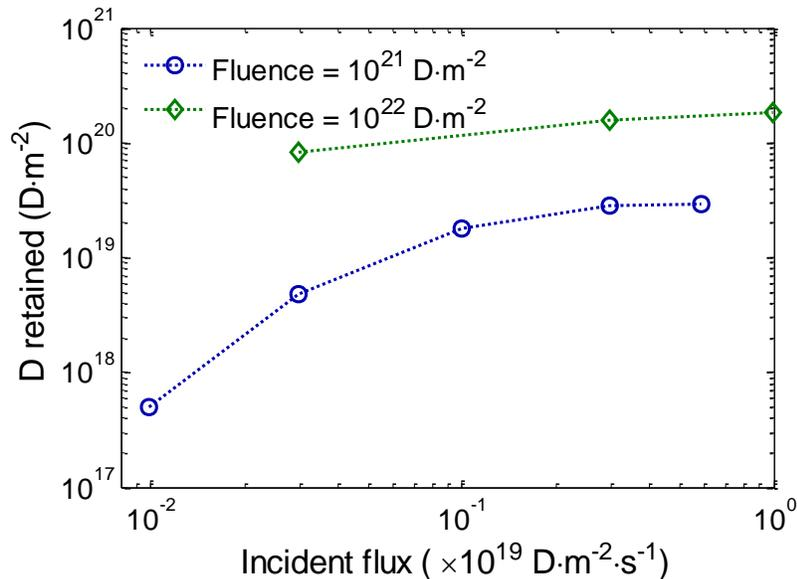
**Figure 2.8.** Evolution of D retention in SCW as function of incident flux [26]. The SCW is implanted with 500 eV/D at fluence of  $10^{21} \text{ D}/\text{m}^2$  and  $10^{22} \text{ D}/\text{m}^2$ . During the implantation, a LN<sub>2</sub> cold trap is used to reduce the amount of impurities in the chamber for the blue data point (fluence =  $10^{21} \text{ D}/\text{m}^2$ ). This LN<sub>2</sub> cold trap is not used for the other set of data (fluence =  $10^{22} \text{ D}/\text{m}^2$ ).
