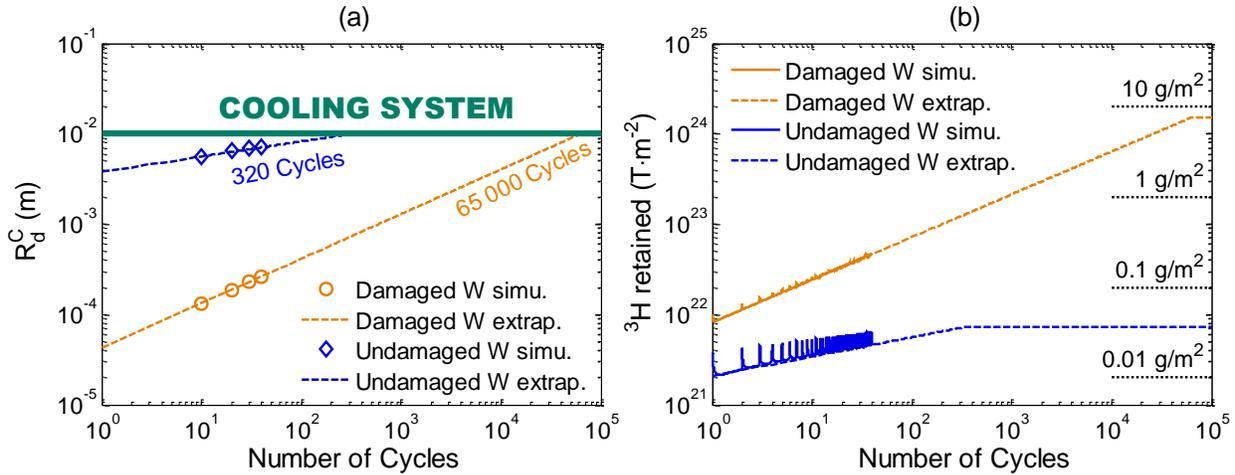
**Figure 5.8.** (a) evolutions of the depth  $R_d^C(N_{\text{cycles}})$  with  $N_{\text{cycles}}$  for undamaged (blue) and damaged (orange) W. The marker corresponds to the value extracted from the simulations and the dashed line corresponds to the extrapolation laws obtained.
