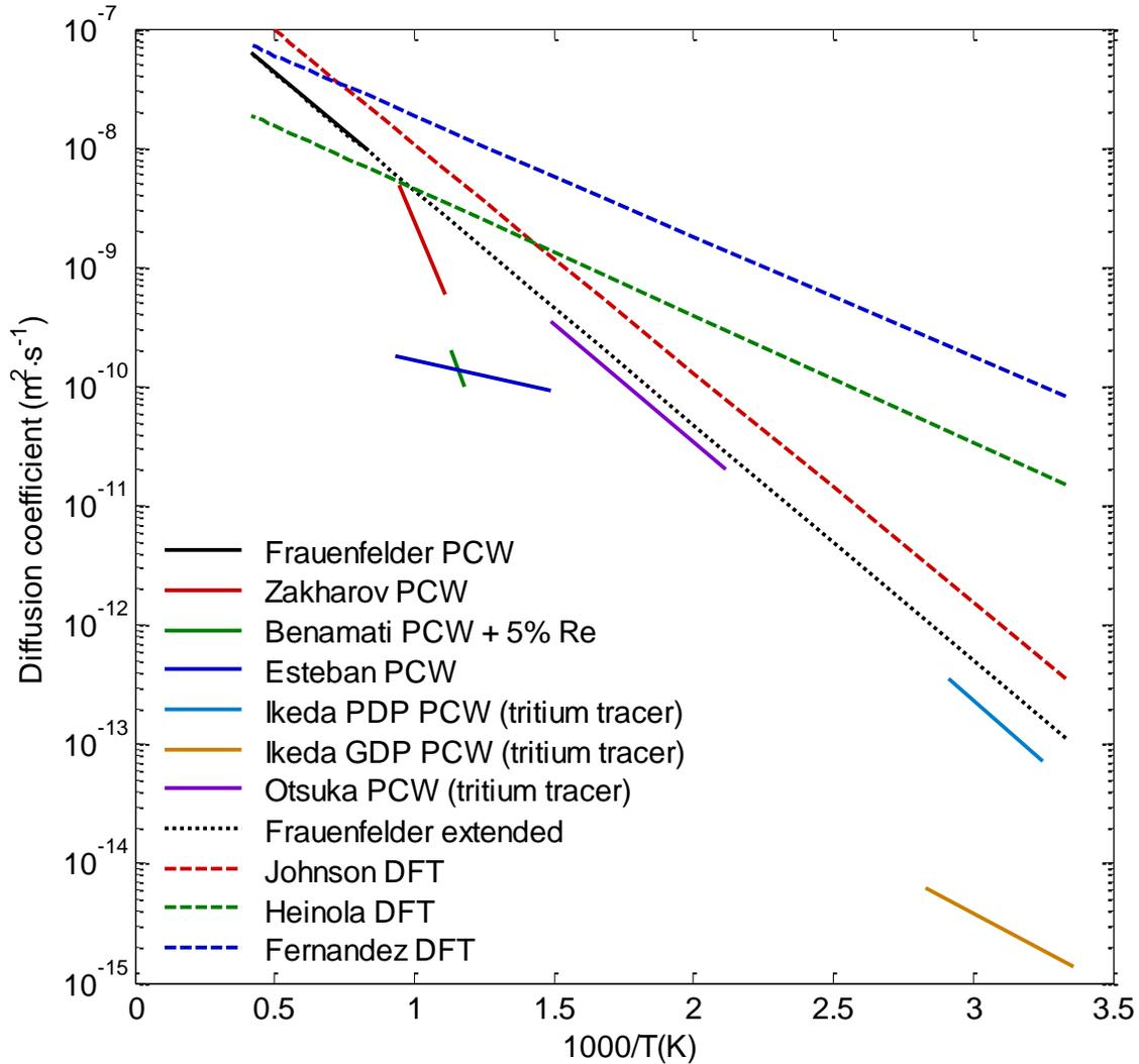
**Figure 2.6.** Temperature dependence of hydrogen diffusion coefficient in W. The solid lines correspond to experimentally determine diffusion coefficient from Frauenfelder [29], Zakharov [81], Benamati [74], Esteban [78] Ikeda [79, 80] and Otsuka [82, 83]. The dotted line corresponds to the extension of Frauenfelder dependence assumed to be the most relevant experimental data. The dashed lines correspond to different theoretical DFT results from Johnson [65], Heinola [71] and Fernandez [72].
