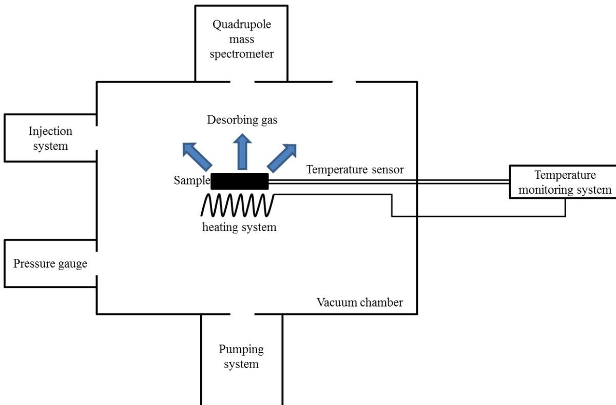
**Figure 2.3.** Schematic description of a standard TDS device.
