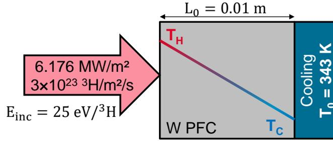
**Figure 5.2.** Simple description of the actively cooled 1-cm-thick W PFC experiencing a heat flux of  $6.176 \text{ MW/m}^2$  and an implanted flux of  $3 \times 10^{23} \text{ }^3\text{H/m}^2 \cdot \text{s}^{-1}$  of  $25 \text{ eV/}^3\text{H}$  ions and cooled at the back side by water at  $T_0 = 343 \text{ K}$ .  $T_C$  is the temperature of the W PFC at the back side where it is cooled and  $T_H$  is the temperature of the W PFC where it receives the heat flux (hot temperature).
