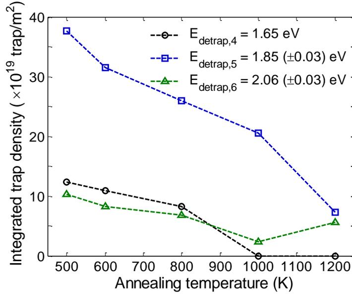
**Figure 4.21.** Integrated amount between 0 and 2.4  $\mu\text{m}$  of the trap concentrations of self-irradiation induced traps as function of the annealing temperature for the simulation of D atom exposure at 500 K. The point at 500 K corresponds to the non-annealed case.
