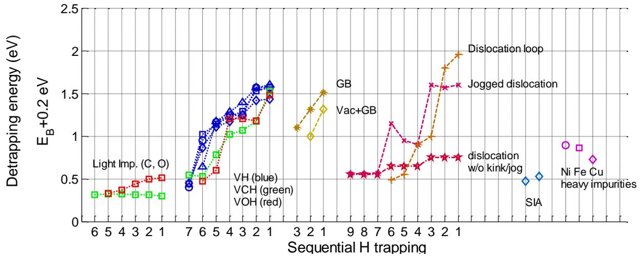
**Figure 2.16.** Non exhaustive overview of detrapping energies calculated by DFT for various types of defects: light C and O impurities, vacancy, Grain Boundary, different type of dislocation, self-interstitial atom and substitutional metallic atom. The sequential H trapping stands for the number of H that is trapped in defect.
