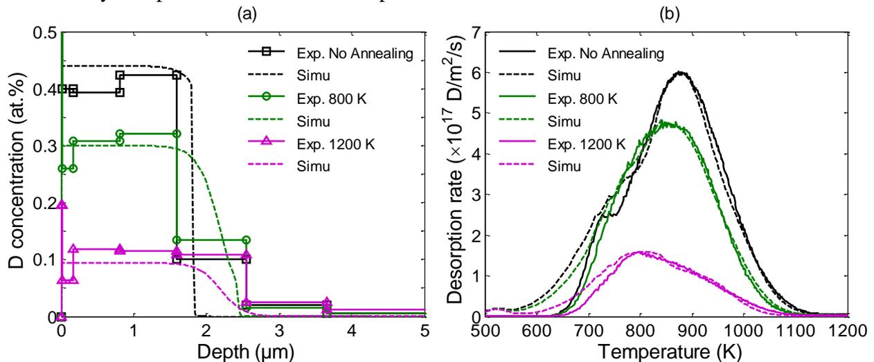
**Figure 4.20.** (a) Comparison between the experimental and simulated D depth profiles obtained after 144 h D atom exposure on self-damaged W samples with a flux of  $2.9 \times 10^{19}$  D $\cdot\text{m}^{-2}\cdot\text{s}^{-1}$  at 500 K.
