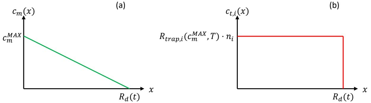
**Figure 3.4.** Simple analytical model describing the concentration of mobile particles (a) and the concentration of trapped particles (b) at a time  $t$  during an atomic exposure.
