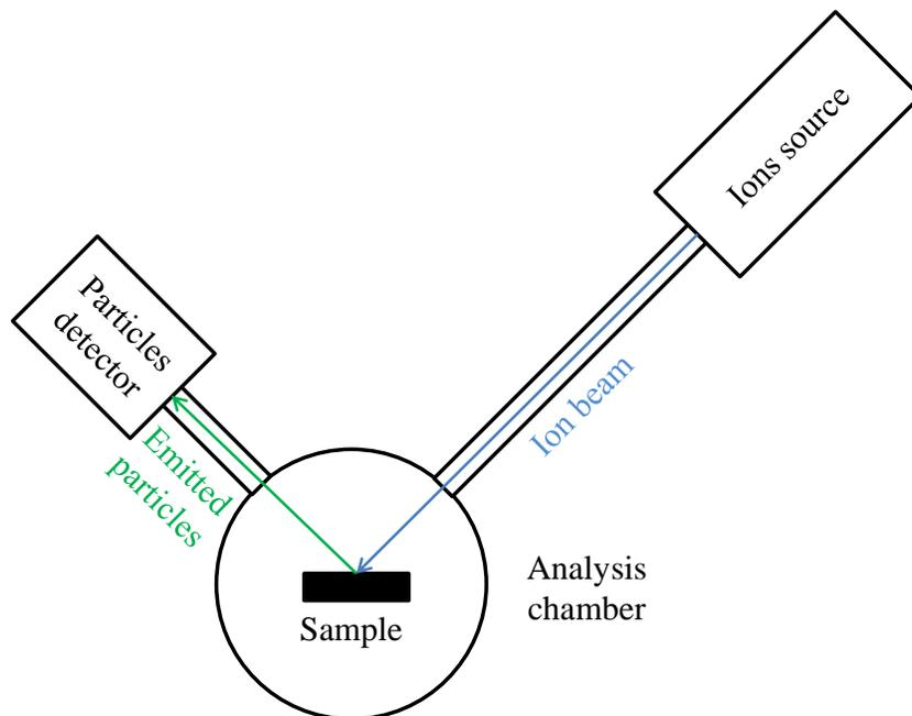
**Figure 2.5.** Schematic description of an IBA device.
