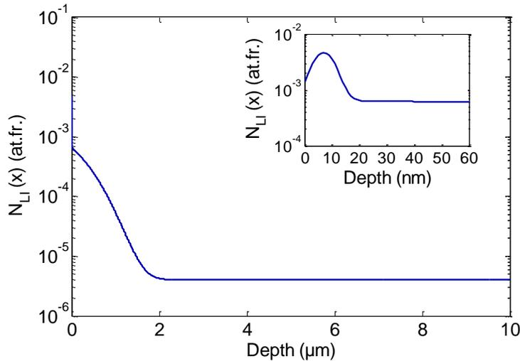
**Figure 4.9.** Distribution  $N_{\text{LI}}(x)$  used in the simulation at high fluence to decrease the trap creation efficiency for depth higher than 1 – 2 μm. The distribution in the first 60 nm does not change compare to the figure 4.2.
