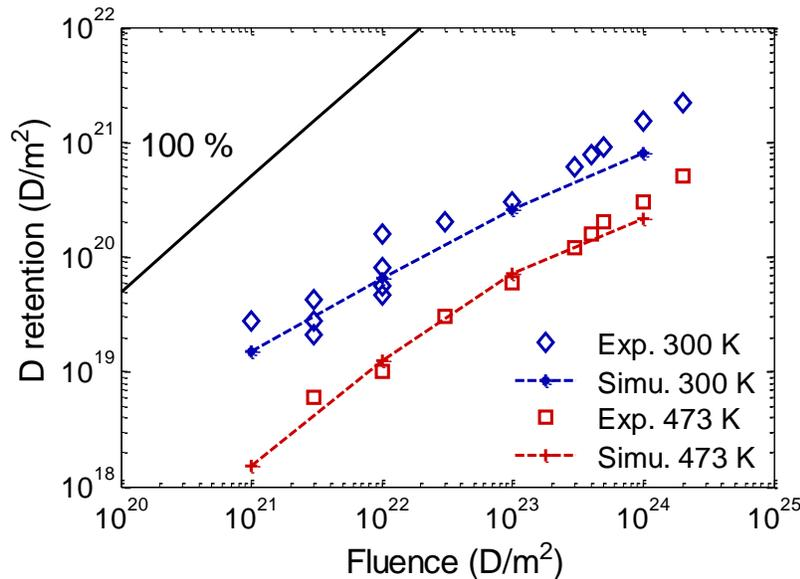
**Figure 4.17.** Evolution of the D retention as a function of the incident fluence for the simulations (dotted line) and the experiments (data points) at 300 K (blue) and at 473 K (red). The incident flux is  $2.5 \times 10^{19} \text{ D} \cdot \text{m}^{-2} \cdot \text{s}^{-1}$  and the ion energy is 200 eV/D. The black solid line corresponds to a full retention of the incident fluence with a reflection coefficient of 0.5.
