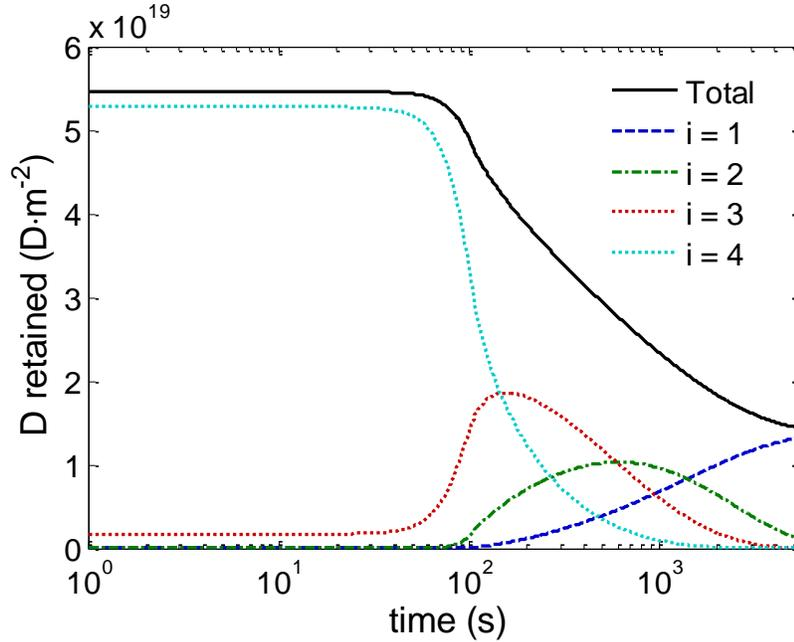
**Figure 4.5.** Evolution of the overall D retained (mobile + trapped) and evolution of the D retained in the traps filled with  $i$  D with  $1 \leq i \leq 4$  during a baking step where the temperature is 400 K for 1.5 h. The time  $t = 0$  s corresponds to the starting of the baking step. The amount of mobile particles and the amount of D trapped in traps filled with 5 and 6 D are not shown because these quantities are too low to be seen.
