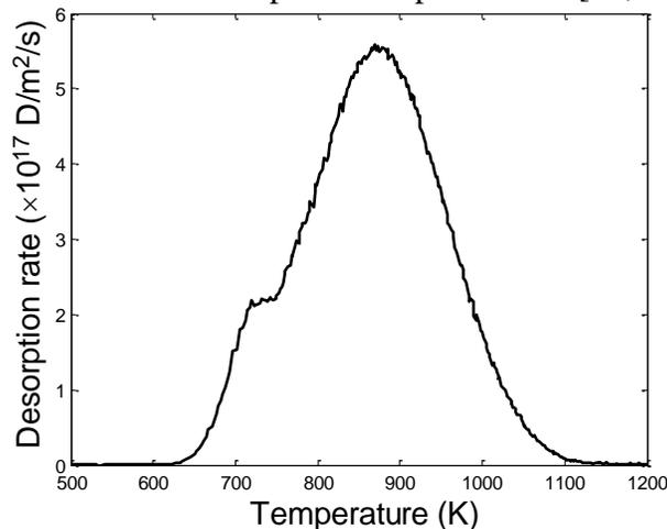
**Figure 2.15.** Experimental TDS spectra obtained with a heating rate of 15 K/min after the exposure on a self-damaged W sample. The damaging is obtained using 20 MeV  $\text{W}^{6+}$  ions and the samples are damaged at 0.5 dpa. These data are from Zaloznik et al. paper [52].
