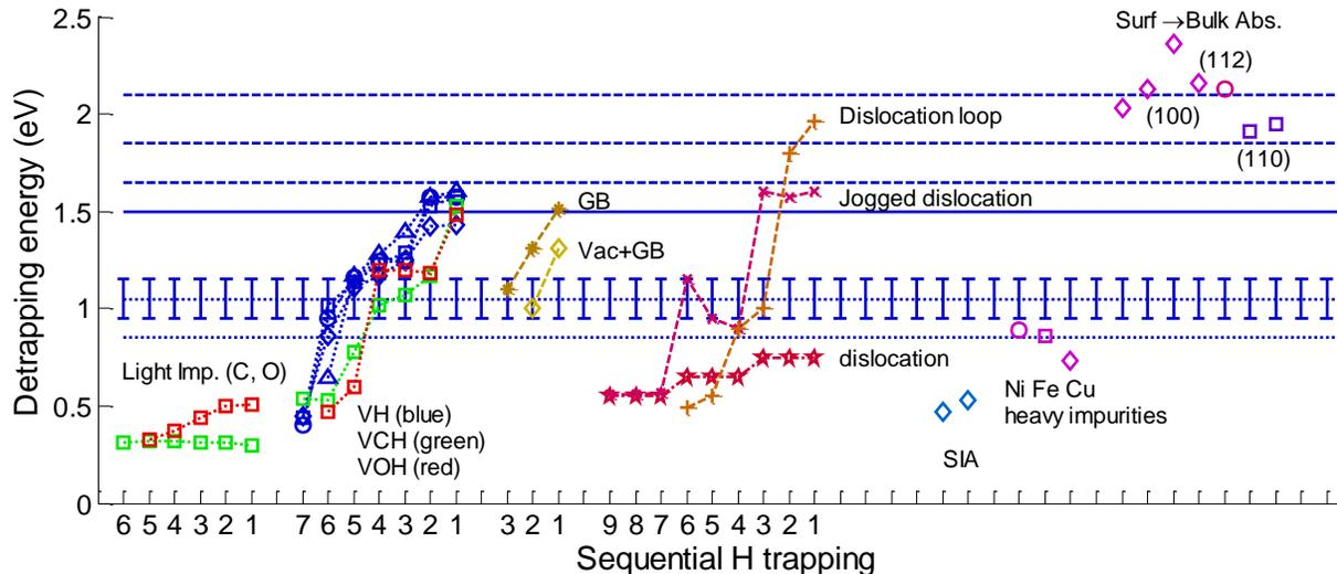
**Figure 4.25.** Comparison between the detrapping energies extracted from DFT ( $E_{\text{Binding}} + 0.2 \text{ eV}$ ) for different defects and the detrapping energies obtained from the simulation of undamaged and self-damaged PCW experiments. The detrapping energies from voids with  $D_2$  are the absorption energies from surface to bulk.
