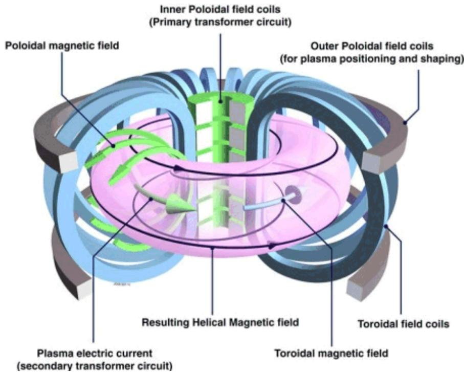
Figure 1.1. Tokamak configuration elements [4]
