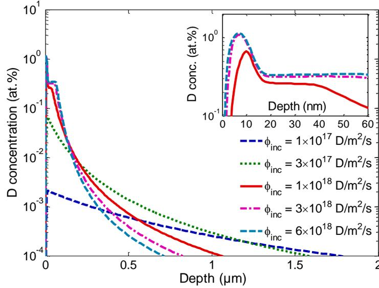
**Figure 4.6.** D Depth profiles obtained for the five simulations of 500 eV/D implantations with five different incident fluxes (from  $10^{17} \text{ D}\cdot\text{m}^{-2}\cdot\text{s}^{-1}$  to  $6\times 10^{18} \text{ D}\cdot\text{m}^{-2}\cdot\text{s}^{-1}$ ) at 300 K. The fluence is  $10^{21} \text{ D}\cdot\text{m}^{-2}$ . The depth profiles are the one obtained after the baking step and before the TDS starts.
