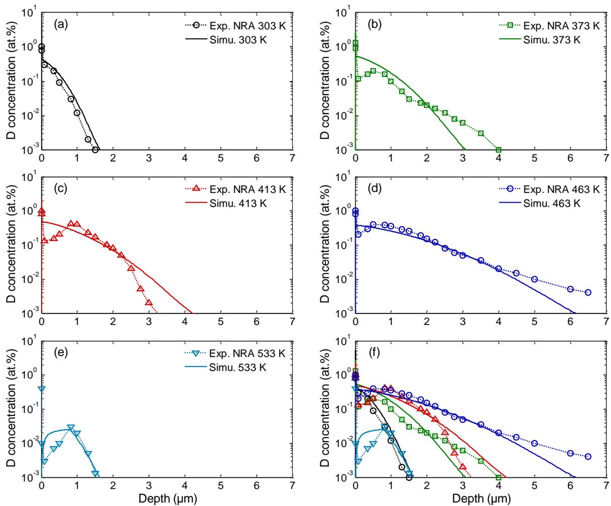
**Figure 4.12.** Experimental (NRA) and simulated D depth profiles obtained after implantation of 500 eV/D ions at an incident flux of  $10^{21} \text{ D}\cdot\text{m}^{-2}\cdot\text{s}^{-1}$  at a fluence of  $2\times 10^{24} \text{ D}\cdot\text{m}^{-2}$  at different temperatures. (a) at 303 K, (b) at 373 K, (c) at 413 K, (d) at 463 K, (e) at 533 K and (f) for all temperatures.
