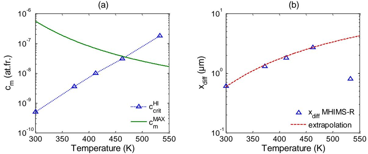
**Figure 4.13.** (a) Evolutions with the implantation temperature of  $c_{\text{crit}}^{\text{HI}}$  and  $c_m^{\text{MAX}}$  for the implantation of 200 eV/D with an incident flux of  $10^{21} \text{ D} \cdot \text{m}^{-2} \cdot \text{s}^{-1}$ .
