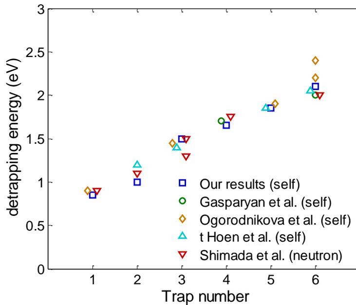
**Figure 4.24.** Detrapping energies obtained from different MRE studies in self-damaged (self) and neutron (neutron) damaged PCW experiments. For our results, the 6 detrapping energies are shown even if trap 3 is not used in our simulations of self-damaged PCW.
