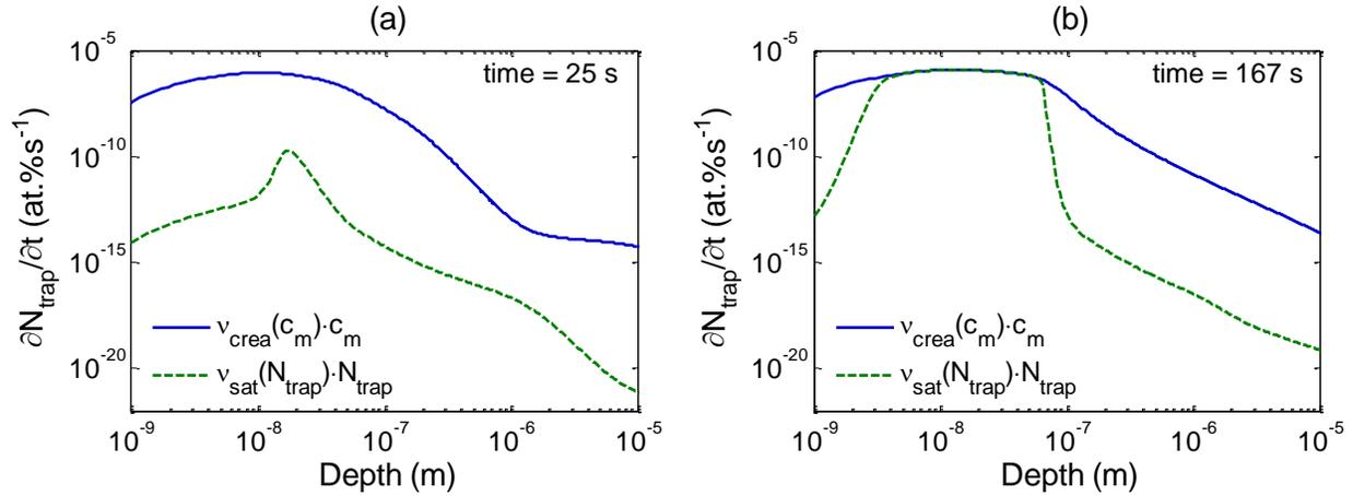
**Figure 4.8.** Depth distribution of  $v_{\text{crea}}(c_m) \cdot c_m$  and  $v_{\text{sat}}(N_{\text{trap}}/N_{\text{LI}}(x)) \cdot N_{\text{trap}}$  at two different times. (a) at  $t = 25$  s in the linear growth regime and (b) at  $t = 167$  s in the saturated regime. The simulated incident flux is  $6 \times 10^{18} \text{ D} \cdot \text{m}^{-2} \cdot \text{s}^{-1}$  and the fluence is  $10^{21} \text{ D} \cdot \text{m}^{-2}$ .
