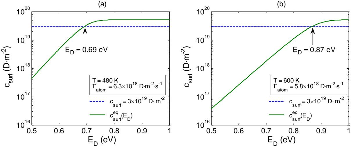
**Figure 4.19.** (a) Green solid line: evolution of  $c_{\text{surf}}^{\text{eq}}$  with  $E_D$  given by equation 3.29 for a temperature of 480 K and an incident flux of  $6.3 \times 10^{18} \text{ D} \cdot \text{m}^{-2} \cdot \text{s}^{-1}$ , Blue dashed line: experimentally measured (ERDA) value of  $c_{\text{surf}}$  in [41] in the same conditions.
