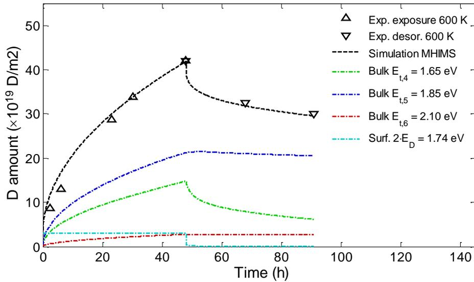
**Figure 4.22.** Comparison between the simulated and experimental evolutions of the D total amounts with time during a 48 h atomic exposure at 600 K with an incident flux of  $5.8 \times 10^{18} \text{ D} \cdot \text{m}^{-2} \cdot \text{s}^{-1}$  followed by an isothermal desorption at 600 K for 43 h.
