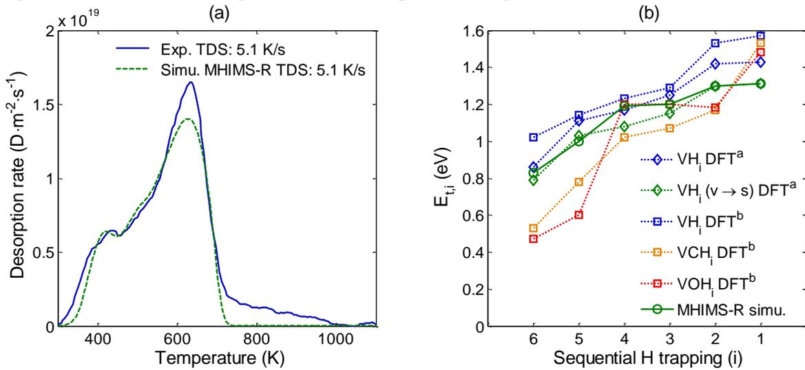
**Figure 4.10.** (a) Experimental (blue solid line) and simulated (green dashed line) TDS spectrum obtained after implantation of 500 eV/D ions in SCW with an incident flux of  $10^{20} \text{ D}\cdot\text{m}^{-2}\cdot\text{s}^{-1}$  and a fluence of  $10^{23} \text{ D}\cdot\text{m}^{-2}$ . The heating rate is 5.1 K/s.
