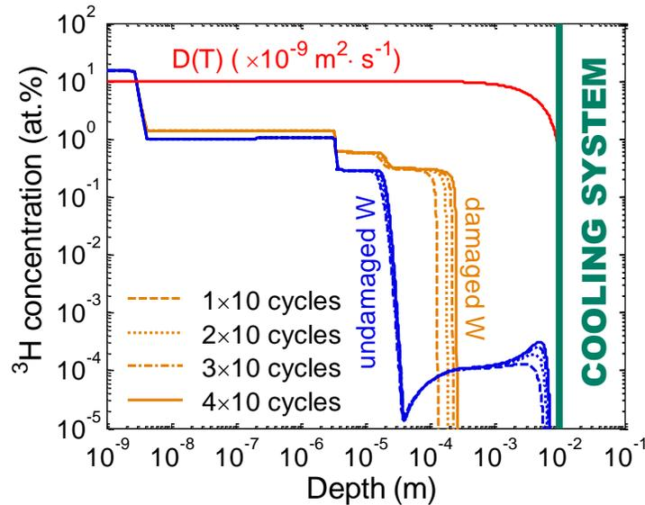
**Figure 5.7.** Simulated  $^3\text{H}$  depth profiles for undamaged (blue) and damaged (orange) W at the end of each group of 10 cycles. The evolution of the diffusion coefficient with depth is also shown in red.
