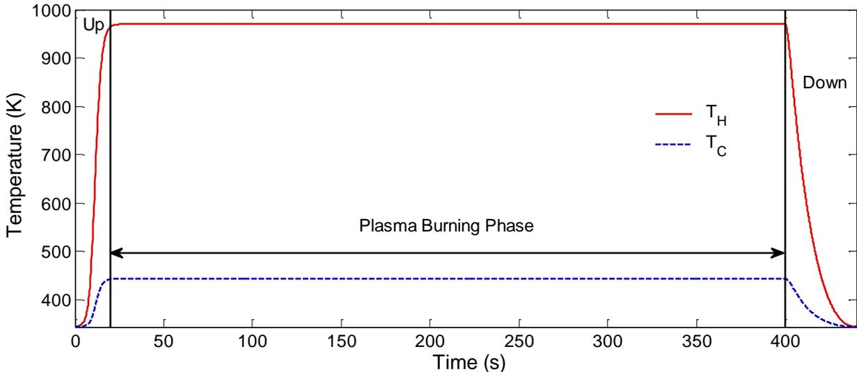
**Figure 5.3.** Evolution of the temperatures of the plasma facing surface ( $T_H$ ) and the cooled surface ( $T_C$ ) during the first three phases (ramp-down, plasma burning, ramp-down).
