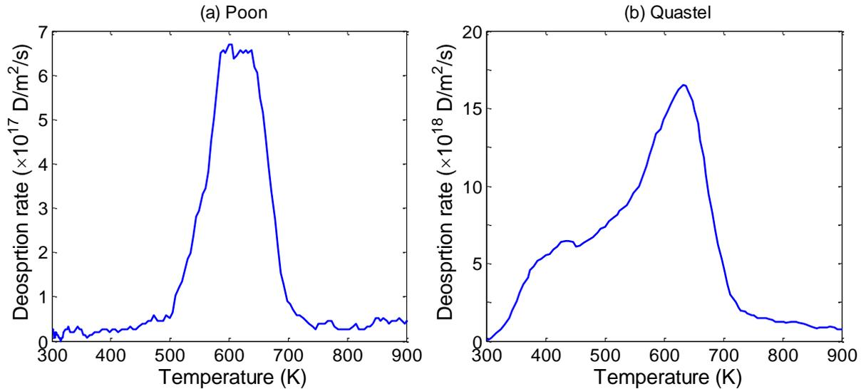
**Figure 2.7.** (a) TDS spectrum after irradiation of SCW at 300 K with D ions at 500 eV/D, flux =  $10^{18}$  Dm<sup>-2</sup>s<sup>-1</sup>, fluence =  $10^{21}$  D/m<sup>2</sup>, heating rate = 4-6 K/s ,(by Poon et al. [26]).
