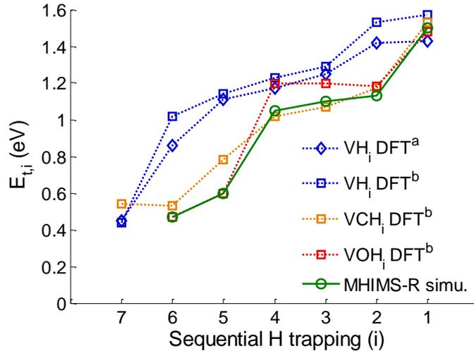
**Figure 4.4.** Detrapping energies as a function of the number of HIs trapped inside the trap. The detrapping energies used in the simulation are compared to detrapping energies calculated by DFT for H in  $VH$ ,  $VOH$  and  $VCH$ . <sup>a</sup> [72], <sup>b</sup> [114].
