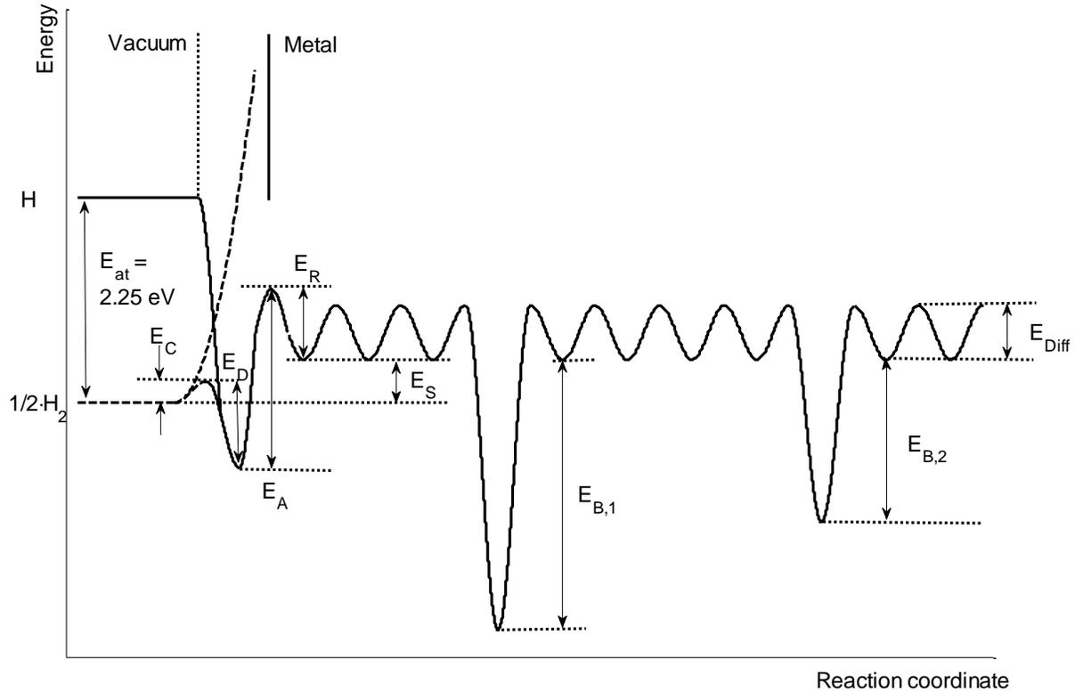
**Figure 2.2.** Schematic idealized energy diagram of H/W interactions. The solid line corresponds to the interactions between H atom and the metal and the dashed line correspond to the interaction between H<sub>2</sub> molecule and the metal.
