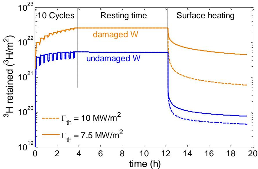
**Figure 5.9.** Evolution of the  $^3\text{H}$  retained with time in damaged (orange) and undamaged (blue) W during 10 cycles followed by a resting time of 11 h and a surface heating with a thermal flux of  $7.5 \text{ MW/m}^2$  (solide line) and  $10 \text{ MW/m}^2$  (dashed line).
