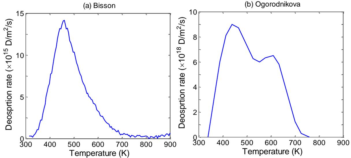
**Figure 2.11.** (a) TDS spectra obtained after irradiation of PCW at 319 K with D ions at 250 eV/D, flux =  $2 \times 10^{16}$  D/m<sup>2</sup>/s, fluence =  $2.9 \times 10^{19}$  D/m<sup>2</sup>, heating rate = 1 K/s (by Bisson et al. [24]).
