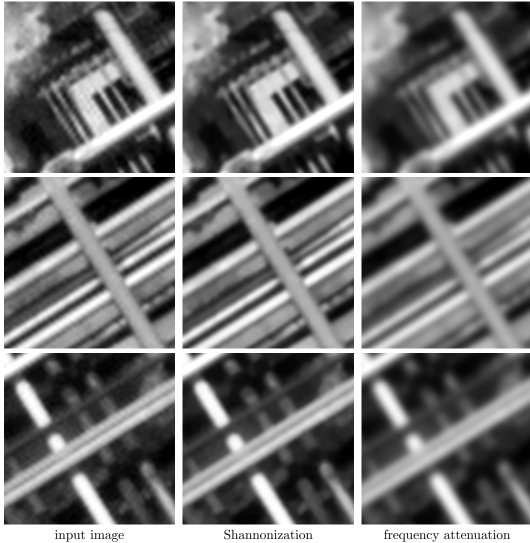
Figure 3.11: Details of Figure 3.10 with Shannon resampling. Different Parts of the three images of the first row of Figure 3.10 are shown after Shannon interpolation. As expected, the output of the “Image Shannonizer” (middle) is well interpolable, contrary to the input image (left) on which oscillations appear. A simple frequency attenuation (right) is not efficient, since it introduces a large amount of undesired blur.
