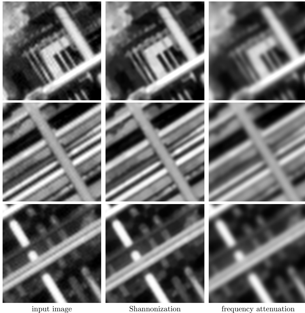
Figure 3.11: Details of Figure 3.10 with Shannon resampling. Different Parts of the three images of the first row of Figure 3.10 are shown after Shannon interpolation. As expected, the output of the “Image Shannonizer” (middle) is well interpolable, contrary to the input image (left) on which oscillations appear. A simple frequency attenuation (right) is not efficient, since it introduces a large amount of undesired blur.
