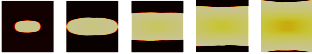
Fig. 3.33: Central stimulus. Case II. \sigma_{l,n}^d = 0.2 . |Y_B| = 0.61 . Observing transmembrane voltage, v at times: 20ms , 50ms , 100ms , 150ms and 200ms .
