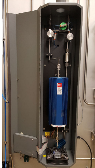
Figure 3.16 – XEMIS1 rare-gas purifier.
