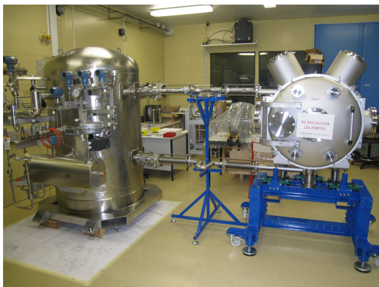
Figure 3.27 – General view of the XEMIS2 experimental set-up installed in Subatech laboratory: right) XEMIS2 cryostat and left) Recovery and Storage of Xenon (ReStoX).
