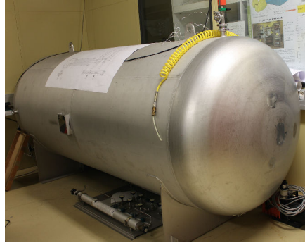
Figure 3.26 – 4\text{ m}^3 rescue tank used to recuperate the xenon in case of emergency.
