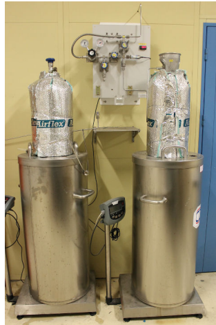
Figure 3.22 – High pressure bottles used to store the gaseous xenon when the detector is not in use.
