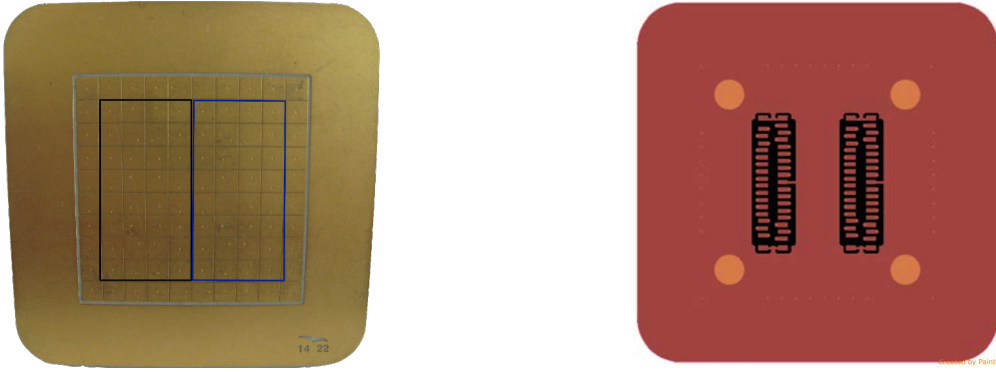
Figure 6.16 – Relative position of the two IDeF-X LXe chips (black and blue line) with respect to the pixels in the anode. In the right figure the location of the connectors directly wire bounded to the 32 pixels of each ASIC is illustrated.
