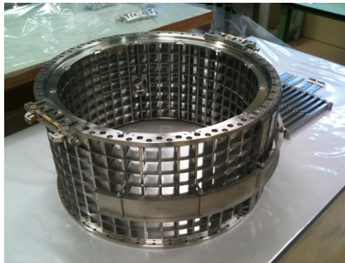
Figure 3.32 – Mounting bracket for the 380 PMTs used to detect the VUV scintillation photons emitted after the interaction of an ionizing particle with the LXe.
