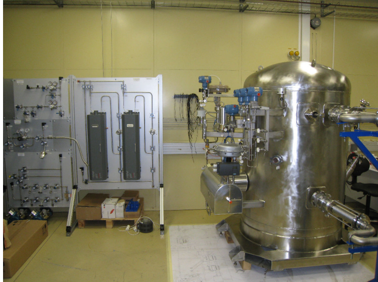
Figure 3.28 – General view of the XEMIS1 experimental set-up installed in Subatech laboratory: right) Recovery and Storage of Xenon (ReStoX) and left) purification system.
