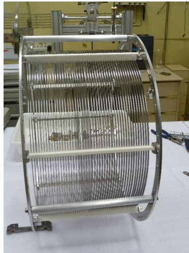
Figure 3.31 – External 46 stainless steel field rings used to provide an uniform electric field along the drift volume of the detector.
