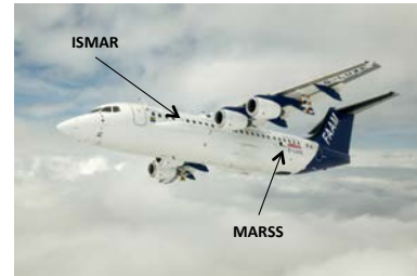
FIGURE 4.2: The positions of ISMAR and MARSS on board the FAAM BAe-146 research aircraft.
