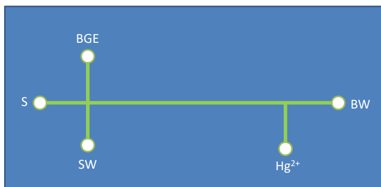
Figure 113: schema of the proposed microchip where an \text{Hg}^{2+} reservoir is added. Separation occurs between S, SW, BGE, and BW reservoirs. Then, potential is applied between S, SW, BGE, and \text{Hg}^{2+} so the RSNOs decompose to nitrite and we detected the different nitrites coming from different RSNOs.
