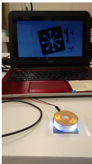
Figure 99: Image of the device connected to laptop by a USB drive which assures lightening. A camera could be connected also to directly analyze the results.
