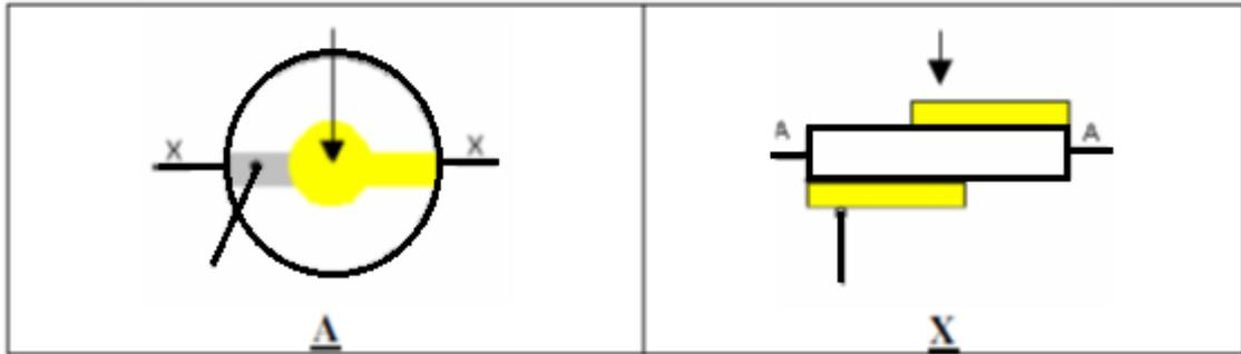
**Figure II-8.** Quartz disk face (A) and cross-sectional (X) carrying the two gold electrodes<sup>109</sup>
