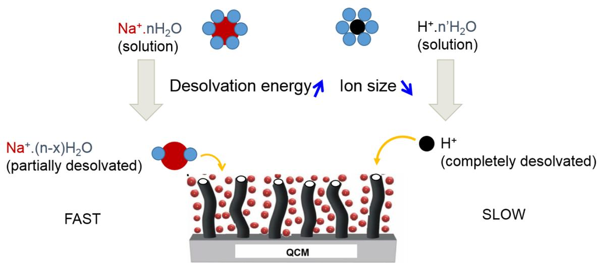
**Figure III-10.** Schematic representation of the interaction of ions with carbon nanotube based electrodes on gold electrodes of the quartz resonator in aqueous 0.5 M NaCl at pH=7.
