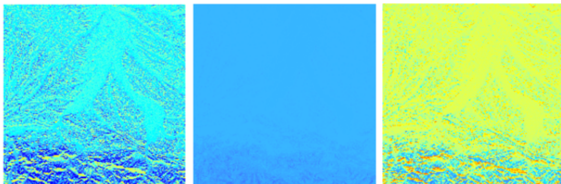
Figure 6.6: Example radiation estimations generated at CESBIO by S.Gascoin. Images correspond to direct, diffuse and total radiation estimations (in WH/m_2 ) for a given tile during the month of January. The range for total radiation in the given example is [0-357383]
