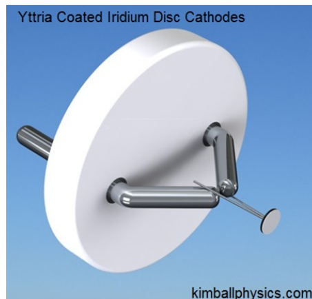
Figure 5.1: Illustration of the yttria-coated iridium disc cathode (modified from [156]).
