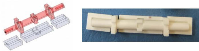
Figure 134: designed and manufactured dielectric part of the filter with support
