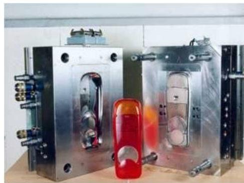
Figure 30: example of mold for injection [34]
