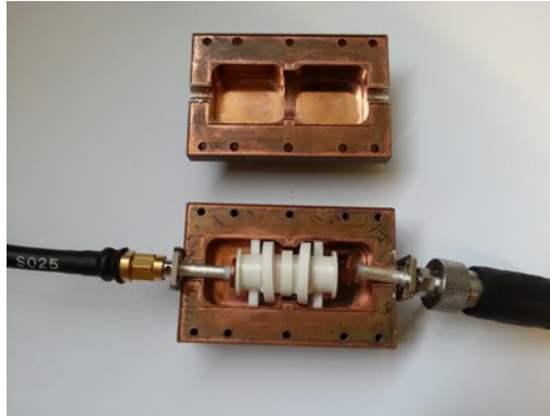
Figure 165: 2-pole filter with tuning system - manufactured elements
