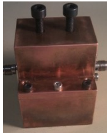
Figure 122: metallic housing for the 2-pole filter
