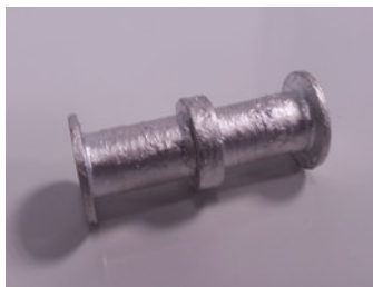
Figure 186: 2-pole dielectric part covered by silver lacquer
