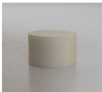
Figure 42: Characterization of the Zirconia material - 4GHz resonator
