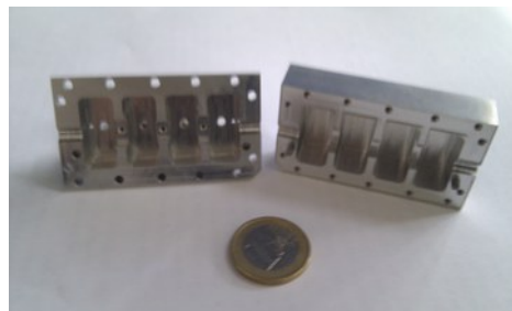
Figure 135: manufactured Aluminum housing for the 4-pole filter
