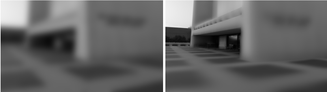
Figure 6.1 – Visual comparison of the uniform Gaussian smoothing (left) and the proposed non-uniform smoothing (right) of the same input image. The latter is propagated “along the surface”: farther objects are less smoothed. An accurate formulation of this principle, referred to as viewpoint covariant behavior , leads to a causal multiscale representation (scale space) allowing for repeatable keypoint detection.
