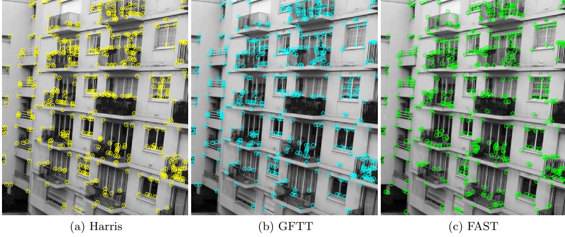
Figure 2.1 – Corners discovered in an image by Harris, GFTT and FAST detectors. 500 corners with the highest score are displayed, OpenCV implementation is used.
