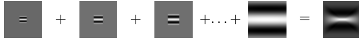
FIGURE 3.7: S1 convolution kernel sum. Kernels smaller than 37 \times 37 are padded with 0's so that they all are 37 \times 37 . Kernels are then summed element-wise so as to produce the kernel on the right. It is worth mentioning the proximity of that kernel with one of the features selected by the Adaboost algorithm in the Viola-Jones framework [30], shown in Figure 3.1.
