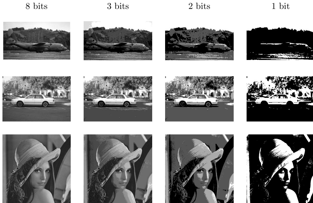
FIGURE 4.2: Precision degradation in input image for three types of objects: faces, cars and airplanes. Color maps are modified so that the 0 corresponds to black and the highest possible value corresponds to white, with gray level linearly interpolated in between. We can see that while the images are somewhat difficult to recognize with 1 bit pixels, they are easily recognizable with as few as 2 bits.
