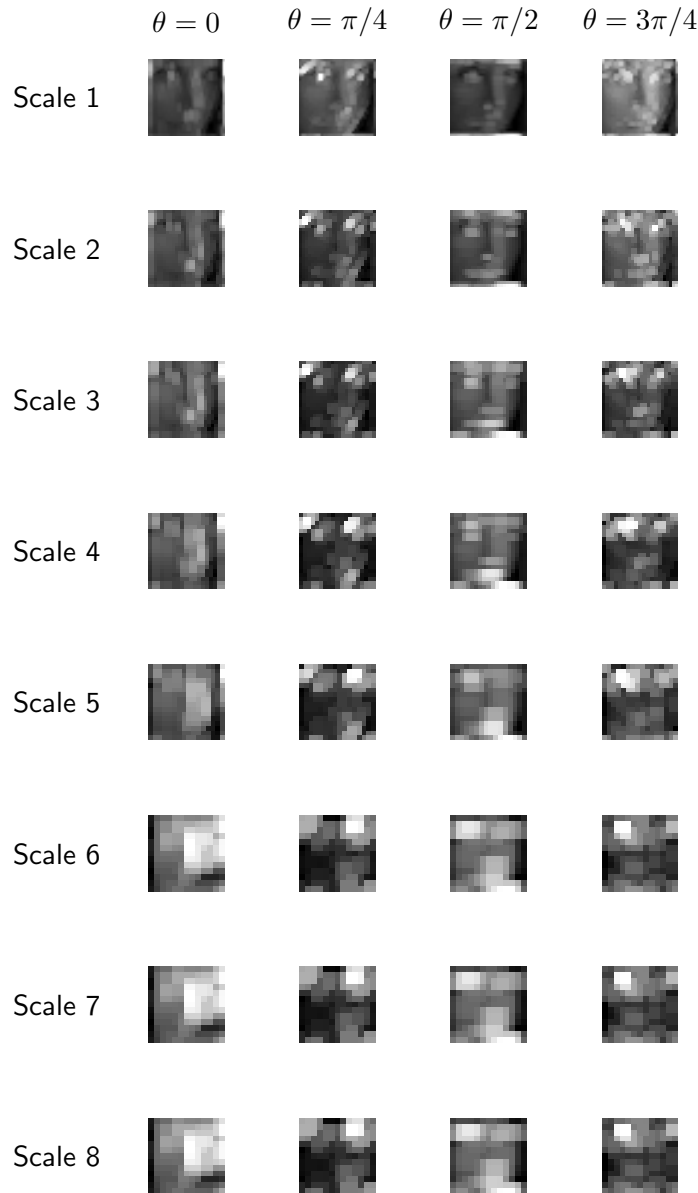
FIGURE 3.6: C1 feature maps for a face. One can see here that most of the features corresponding to an actual feature of a face, e.g the eyes or the mouth, is given by the filters with orientation \theta = \pi/2 .
