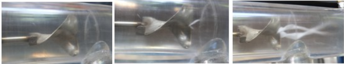
Fig. 5-5: Cavitating vortex stages: A1 no vortex (left), A2 incipient vortex (center), A3 developed vortex (right)
