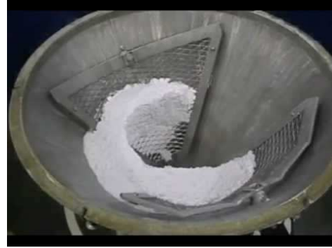
Figure 1.4 – Segregation inside a hopper near the exit hole
