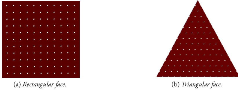
Figure 7.4 – Layout of boundary CP on: (a) rectangular face and (b) triangular face.
