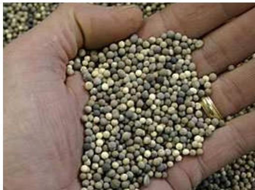
(a) Example of spherical catalyst particles. Credits: Falmouth Products Inc., Falmouth, MA.
