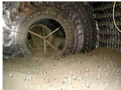
Figure 1.2 – Inside a cement mill
