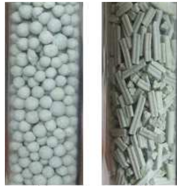
(b) Example of catalyst particles developed at IFPEN.
