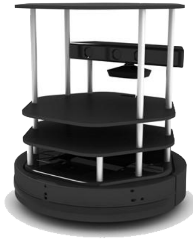
Figure 7.12: TurtleBot kit [ROS 2016a]. Reprinted from "TurtleBot 2, Open-source robot development kit for apps on wheels", from http://www.turtlebot.com/ .
