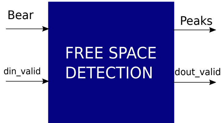
Figure 6.34: External view of free space module.
