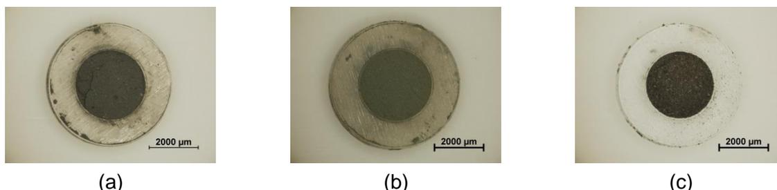
Figure IV.8 : (a) Porte charge Al / CuO ; (b) Porte charge Al / Bi<sub>2</sub>O<sub>3</sub> ; (c) Porte charge ZPP [IV.1].
