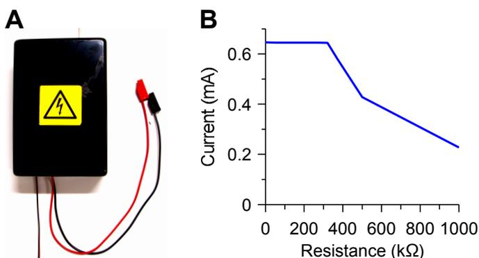
**Figure 7.4 | Reproducible foot shock delivery.** **A** | Custom-built controller used to provide scrambled foot shocks to mice during fear conditioning. **B** | The internal current source provided constant current up to 320 kΩ of body resistance.
