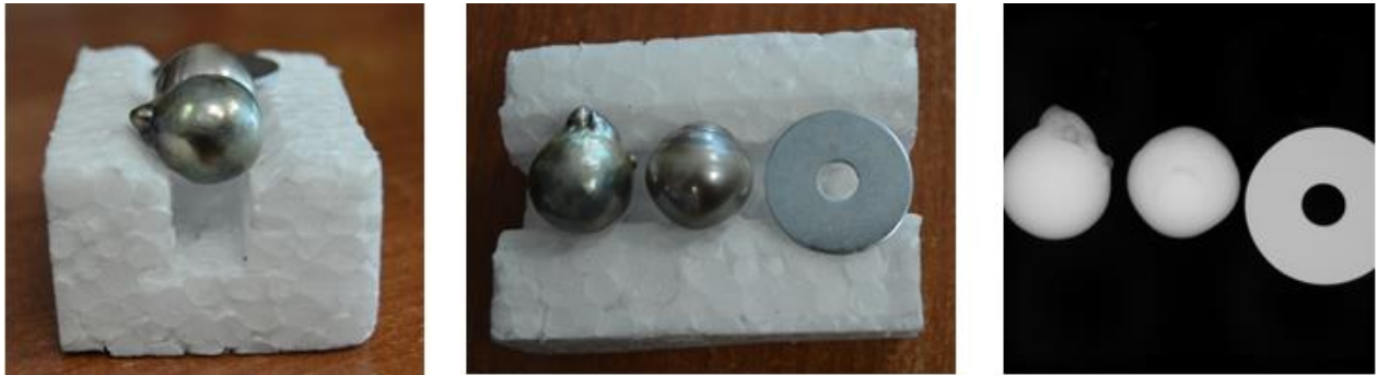
Figure 45: A linear imitation of the borehole geometry with polystyrene and the resulting X-ray image.
