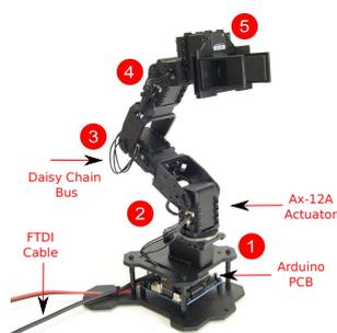
Fig. 5.3 Manipulateur low-cost
