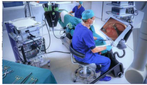
Figure 2.13: TeleFLEX system by the University of Twente. The (green) steering modules are attached to the conventional flexible system (e.g. Anubis) (photo: demcon.nl).
