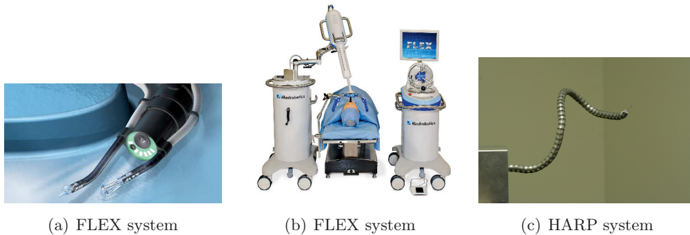
Figure 2.14: The FLEX system in (a) and (b) is composed by an endoscope and two working channels where specific instruments can be inserted (photos: medrobotics.com). The scope is self supporting and take inspiration from the HARP system in (c) (photo:carnegie mellon.)
