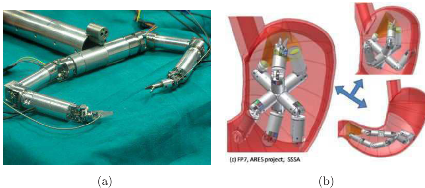
Figure 2.10: In (a) another example of robot for single port surgery (ARAKNES SPRINT, photo: sssa.bioroboticsinstitute.it ). In (b), the concept of ARES project is shown: a miniature-modular robot able to reassemble once got to the desired site inside the human body (photo: Scuola Superiore Sant'Anna).
