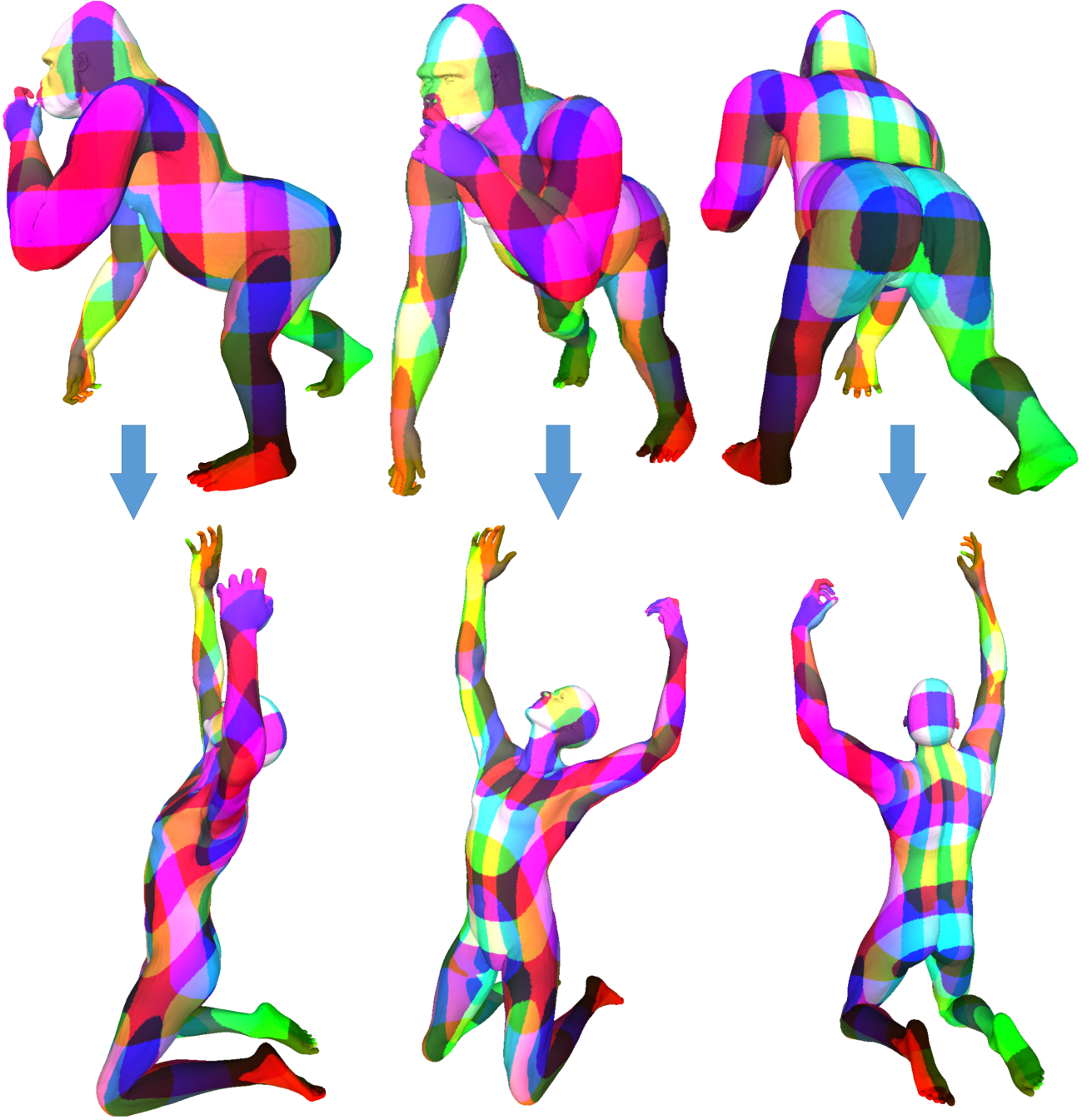
Figure 7.6: Non-isometric mapping. An area relaxation (factor of 10) is used, along with 4 constraints (one at the extremity of each limb) to map the two very different shapes of a gorilla and a man. Requiring more relaxation to better improve the map further would face very slow convergence.
