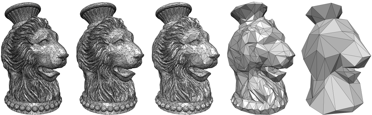
Figure 3.4: Vase Lion. From top left to bottom right: \delta is set to 0.2, 0.3, 0.5, 2.5, and 6.0. The final vertex count is 17,723, 11,042, 6,127, 637 and 109, respectively. The input model is a surface triangle mesh of the vase lion model with 200k vertices.
