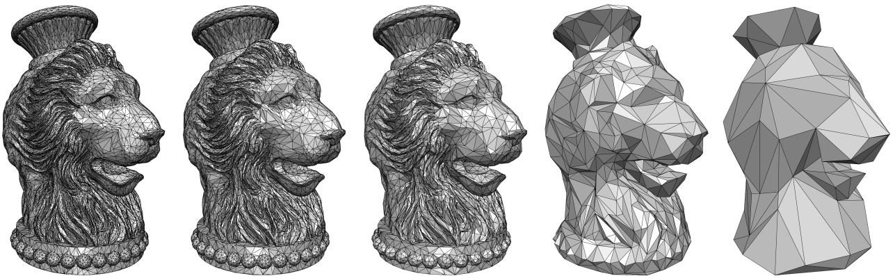
Figure 3.4: Vase Lion. From top left to bottom right: \delta is set to 0.2, 0.3, 0.5, 2.5, and 6.0. The final vertex count is 17,723, 11,042, 6,127, 637 and 109, respectively. The input model is a surface triangle mesh of the vase lion model with 200k vertices.
