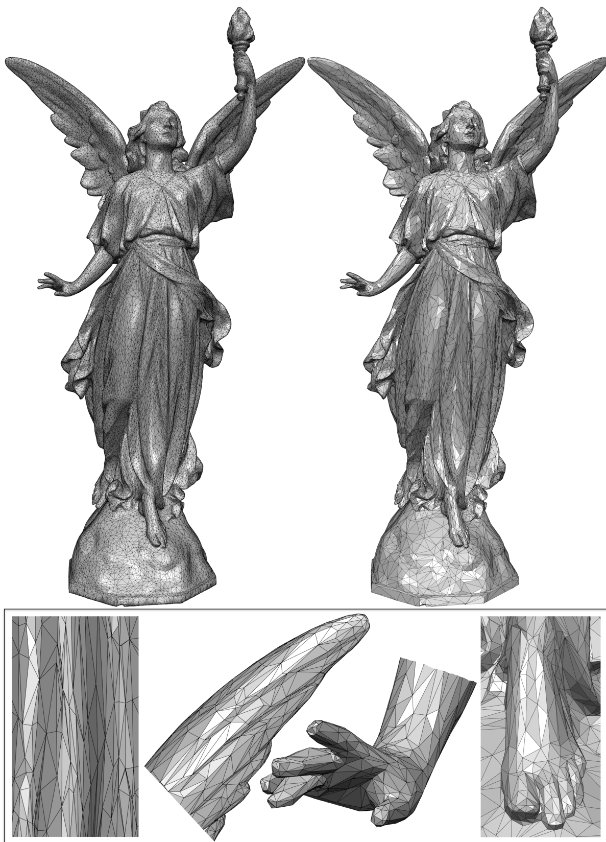
Figure 3.11: Lucy. Left: Input model (50k v ). Right: Output from our algorithm (16.7k vertices, \delta = 0.13\% ).
