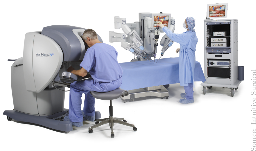
Figure 2.4: Da Vinci surgical system. The surgeon sits at a console and remotely drives a robot to perform the operation.
