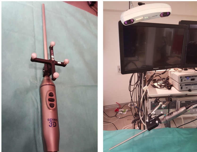
Figure B.1: Optical tracking. On the left, reflective beads are fixed in a pattern and attached to the tracked element, here a laparoscope. On the right, a device with two dedicated cameras is placed in the OR and detects the infrared reflections emitted by the beads for triangulation of the laparoscope's position.
