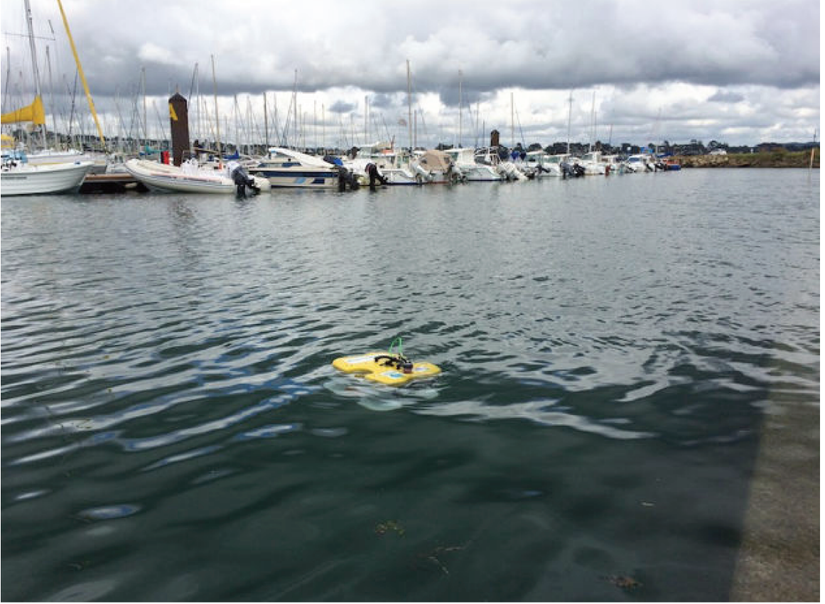
Figure 6-17: The sea experiment of the fully compensated H_\infty heading control approach as well as other control methods on the CISCREA AUV near the Brest harbour, France.
