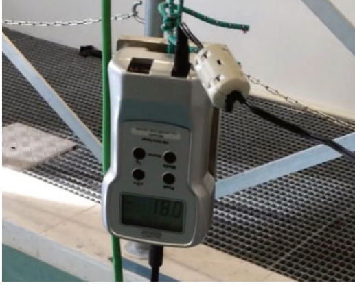
Figure 4-2: Force measurement using a dynamometer with an accuracy of 0.01 N
