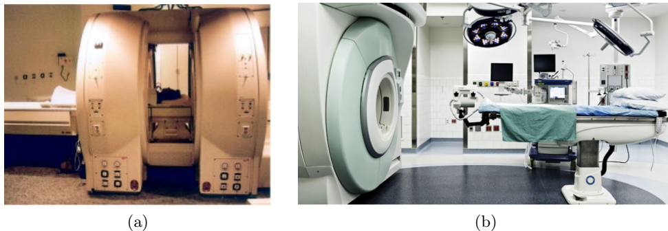
FIGURE 2.8 – Machines IRM peropératoire. (a) IRM bas champ (0.15 T). (b) IRM haut champ (3 T). Illustrations : [Nimsky 2011] (bas champ) et Anton Grassl (haut champ).
