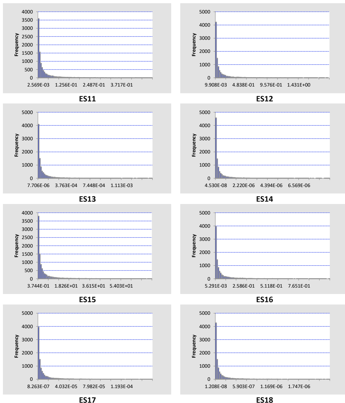
Figure A6-4 Results of the monte carlo simulations for estimating the benchmark dose response in humans ( BMC_h ). The y-axis represents the number of monte-carlo simulations and the x-axis is a unitless dimension of risk, whereby the existence of risk is any value \geq 1 .
