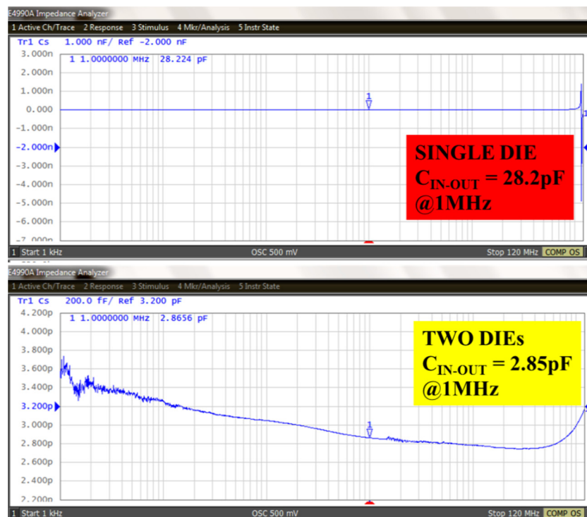
Fig.III.67 Input - output parasitic capacitance of two prototypes
