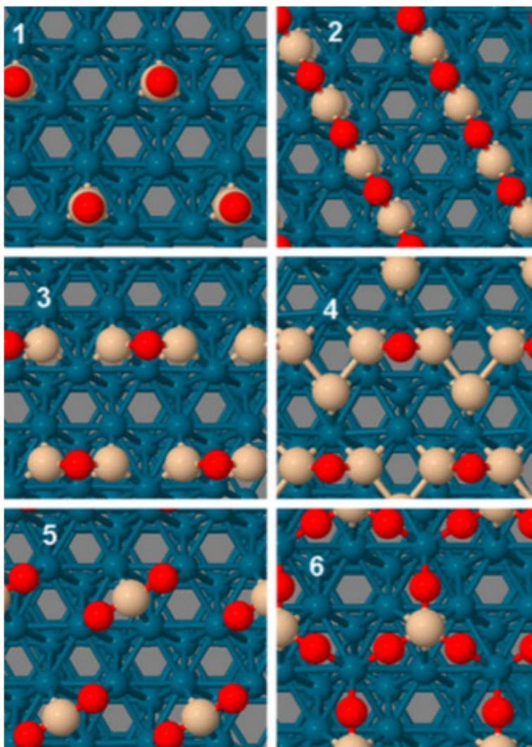
Figure 4.5: (a) RHEED pattern obtained from Si deposited  $(2 \times 2) - 30$  surface. (1-6) models of oxygen (red) and silicon (yellow) forming a  $(2 \times 2)$  structure on the Pd(111) surface are shown, adapted from [48].
