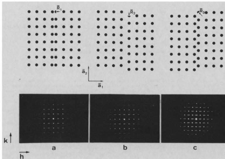
Figure 3.9: Three  $8 \times 8$  dot arrays containing one anti-phase domain boundary. The displacements are marked as  $R_1$ ,  $R_2$  and  $R_3$ . The corresponding diffraction patterns with split diffraction spots are seen in the lower panel. Adapted from [108].
