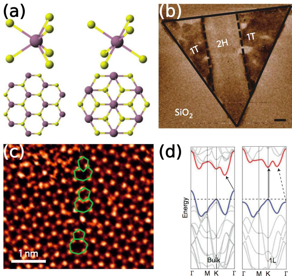
Figure 1.4: Transition metal dichalcogenides. (a) 2H (left) and 1T (right) phases of MoS<sub>2</sub>, (b) Electrostatic Force Microscopy on MoS<sub>2</sub> flake showing 2H (bright) and 1T (dark) regions, (c) a dislocation boundary in MoS<sub>2</sub>, (d) Electronic band structure in bulk (left) and monolayer (right) of MoS<sub>2</sub>. Adapted from [17] [131].
