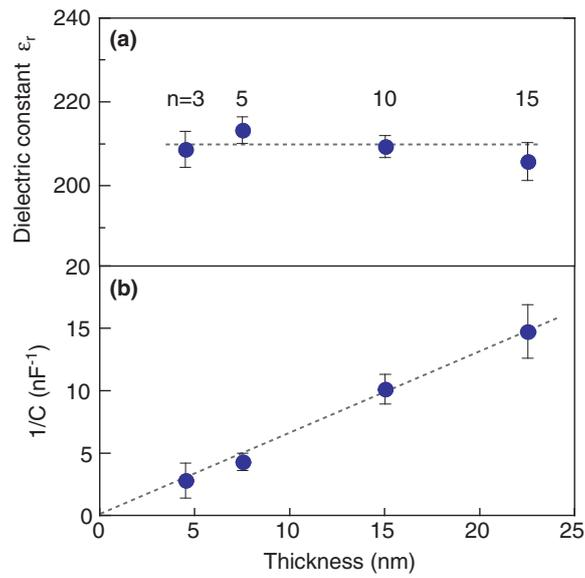
Figure 1.7: (a) The dielectric constant value as a function of thickness of  $(\text{Ca}_2\text{Nb}_3\text{O}_{10})_n$  film. The dielectric constant value does not change on varying the thickness. (b) The reciprocal capacitance from ultra thin films of oxide is a linear function of the thickness that passes through a zero value showing no charge due to a dead layer commonly observed on bulk dielectrics [81].
