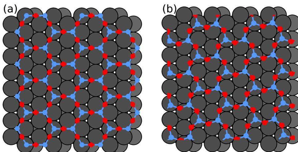
Figure 4.12: (a) Monolayer silicon oxide on Ru(0001). (b) Monolayer silicon oxide on Ru(0001) with rotated [SiO<sub>4</sub>] tetrahedra due to compression as predicted in [7] [2].
