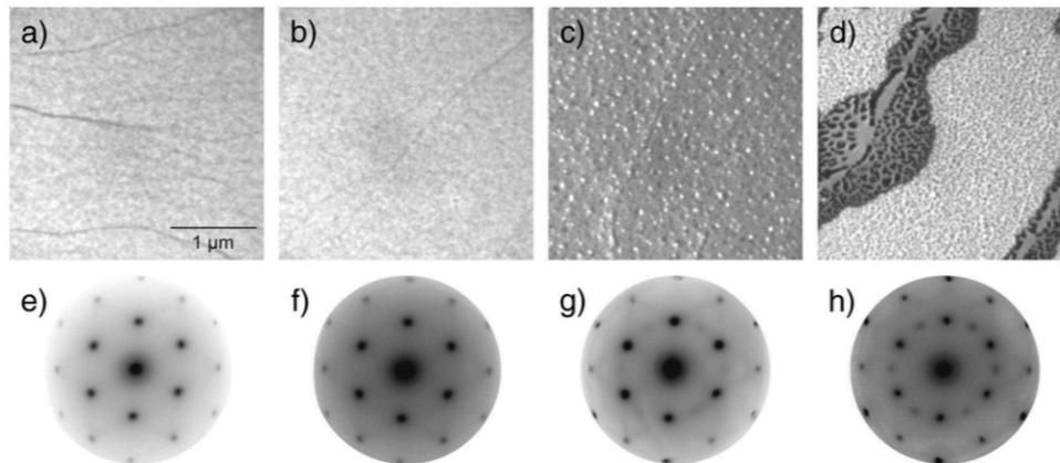
Figure 1.32: LEEM images and corresponding LEED patterns after post-oxidation of bi-layer silicon oxide on Ru(0001) at (a, e) 995 K, (b, f) 1045 K, (c, g) 1095 K and (d, h) 1270 K. Adapted from [52].
