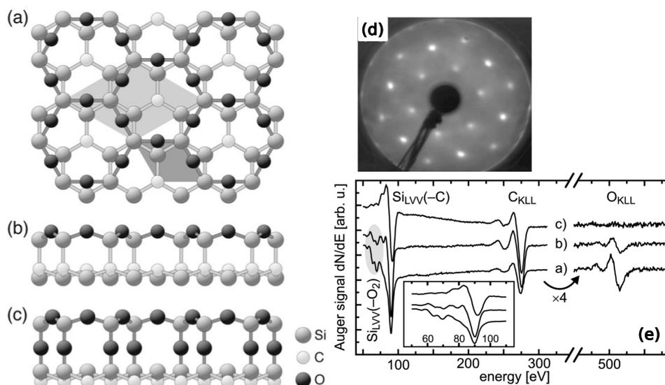
Figure 1.14: (a) ML-Silicon oxide grown on SiC surface. The monolayer depicts a  $R30^\circ$  reconstruction in respect to SiC surface; LEED in (d). Two different phases, one with Si-O-Si on silicon face (b) and Si-O-Si on carbon face (c) on the SiC crystal. (e) Corresponding Auger spectra. Adapted from [8].
