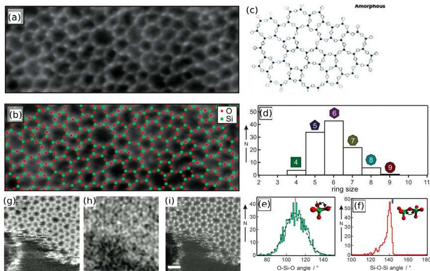
Figure 1.24: Random network of silica rings. (a) STM image ( $8 \text{ nm} \times 3 \text{ nm}$ ) at 100 mV and 100 pA. (b) Ball model overlaid image of (a). (c) Random network model predicted by Zachariassen. (d) Ring size distribution, (e) O-Si-O bond angle distribution and (f) Si-O-Si bond angle distribution in (a). (g-h) HREELS maps of silicon and oxygen and (i) ADF image of the amorphous silicon oxide in the same region. Adapted from [64] [42].
