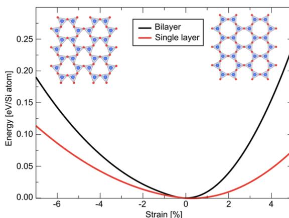
Figure 1.27: Energy-strain curve for monolayer and bilayer silicon oxide. Adapted from [7].
