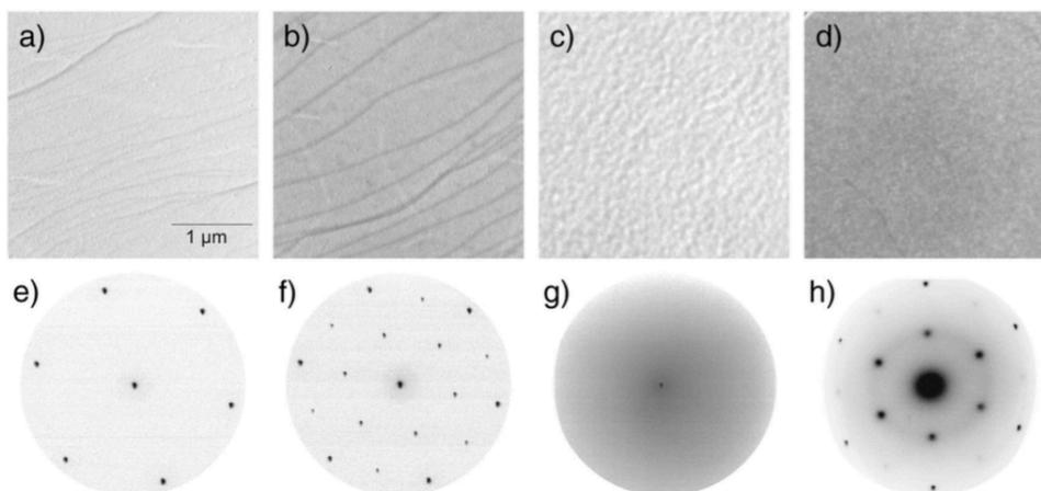
Figure 1.30: LEEM and LEED study during different steps during the growth of bilayer silicon oxide by post-oxidation. (a, e) bare Ru(0001), (b, f)  $(2 \times 2)$ -3O/Ru(0001) reconstruction, (c, g) Si deposition and (d, h) post-oxidation. Adapted from [52].
