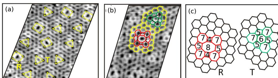
Figure 1.20: (a) An array of T- and R- defects on monolayer silicon oxide grown on Ru(0001) forms on subjecting the monolayer to vacuum annealing. (b) The T- and R- defects are found in vicinity of each other. (c) R- (left) and T- (right) defect structure. Adapted from [119].
