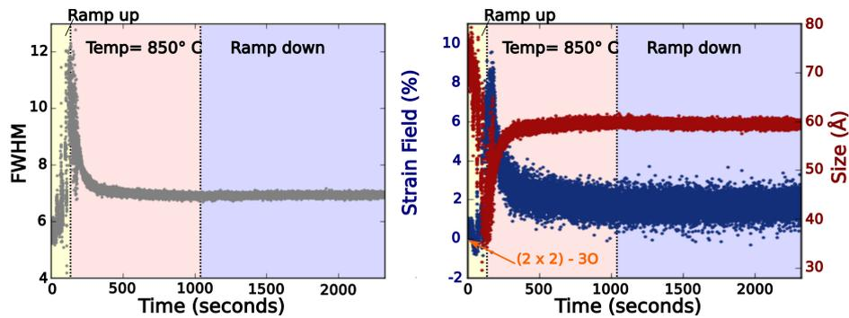
Figure 4.9: (a) FWHM of the silicon oxide streak extracted from gaussian fits and (b) corresponding strain field and domain size as function of time at different temperature. The orange arrow marks the strain field (0%) expected in the  $(2 \times 2) - 30$  domains.
