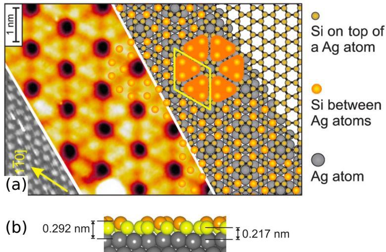
Figure 1.3: Structure of silicene on Ag(111): (a) Top view, (b) Side view. Adapted from [110].
