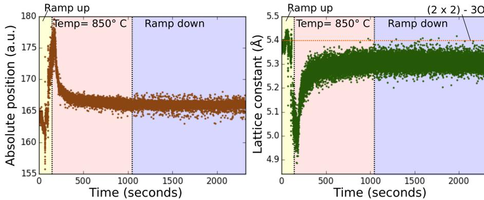
Figure 4.8: (a) Absolute position of the reconstruction streak in reference to specular streak extracted from gaussian fits and (b) the corresponding lattice parameter of monolayer silicon oxide as a function of time.
