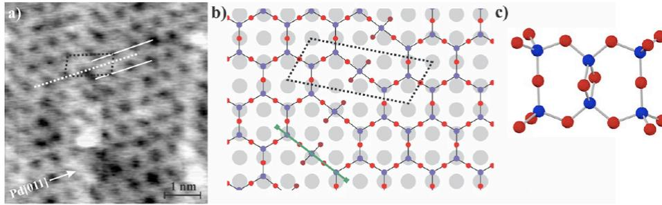
Figure 1.23: Anti phase domain boundary in bilayer silicon oxide on Pd(100) formed by excess of  $[\text{SiO}_4]$  tetrahedra, (a) STM image, (b) ball model of bilayer silica on Pd(100) and (c) cross-sectional model of boundary. Adapted from [2].
