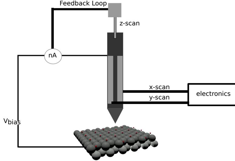
Figure 2.2: The schematic diagram of scanning tunnelling microscope.
