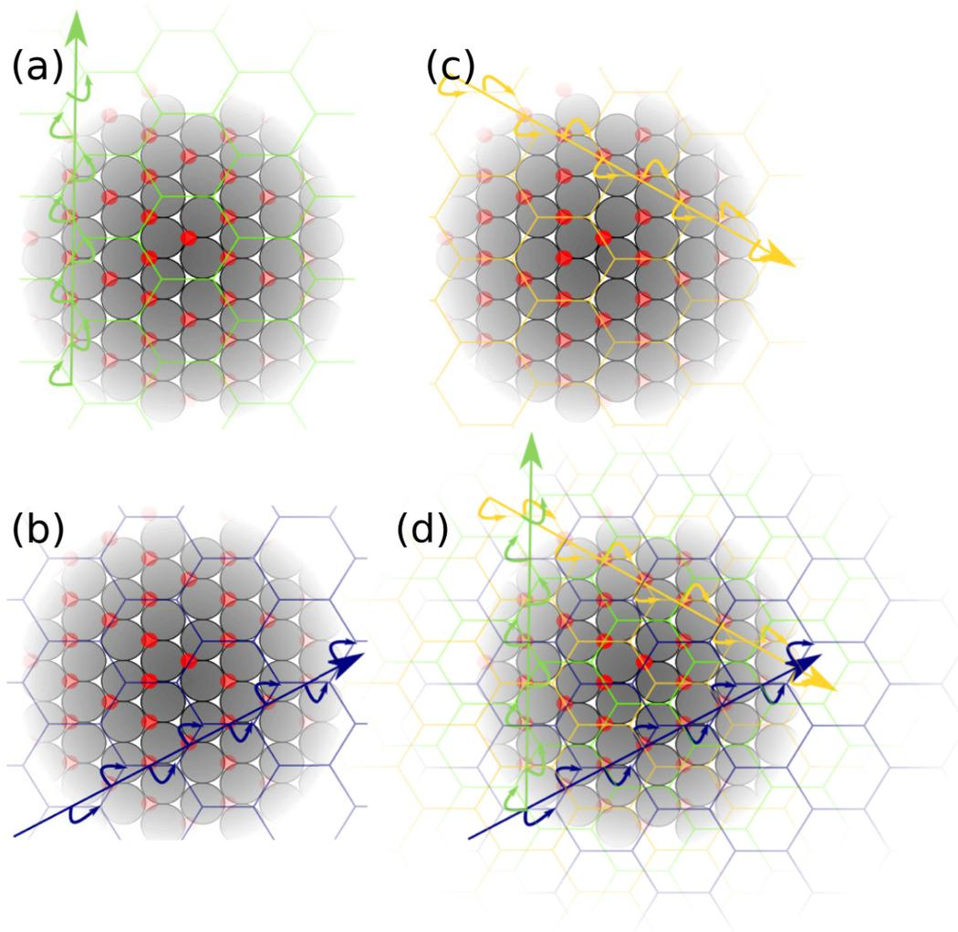
Figure 4.14: (a-c) Translative recrystallisation mechanism of the formation of monolayer silicon oxide in three direction leads to formation of anti phase domains whose mutual shifts are evident by overlapping the three kinds of domains (d).
