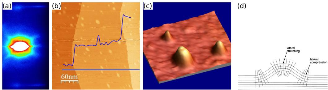
Figure 2.8: (a) RHEED pattern after flash annealing at  $1200^\circ$  and (b) STM image of clean Ru(0001) surface. (c) 3D view and (d) schematic of the argon bubbles. The schematic was adapted from [38].
