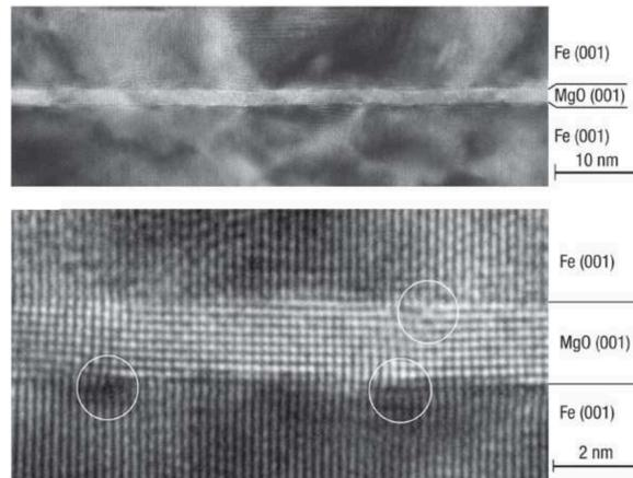
Figure 1.6: Magnetic tunnel junction (MTJ) formed of ultra thin crystalline MgO films sandwiched between two ferroelectric electrodes of Fe. The cross-sectional transmission electron microscopic image shows the crystalline interface between the oxide and the electrodes. Adapted from [126].
