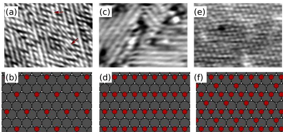
Figure 4.4: STM images and ball-models of various oxygen phases on Ru(0001): (a-b)  $(2 \times 2)$  – O/Ru(0001) mixed with few atom long fragments (exposure of Ru(0001) to 2.5L) (1.4V, 1.7nA). The red arrows mark the nucleation of the  $(2 \times 1)$  reconstruction. (c-d)  $(2 \times 1)$  – O/Ru(0001) (2V, 2nA) (exposure of Ru(0001) to 5L), (e-f)  $(2 \times 2)$  – 3O/Ru(0001) (2V, 0.9nA)(exposure of Ru(0001) to 900L).
