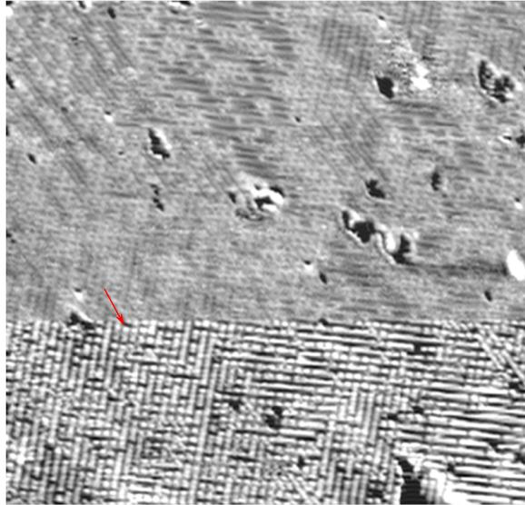
Figure 2.4: Change of tip middle of the scanning on  $(2 \times 1)$  oxygen reconstruction on Ru(0001). The angle between the dense O rows is not  $120^\circ$  as it is expected, due drift during imaging.
