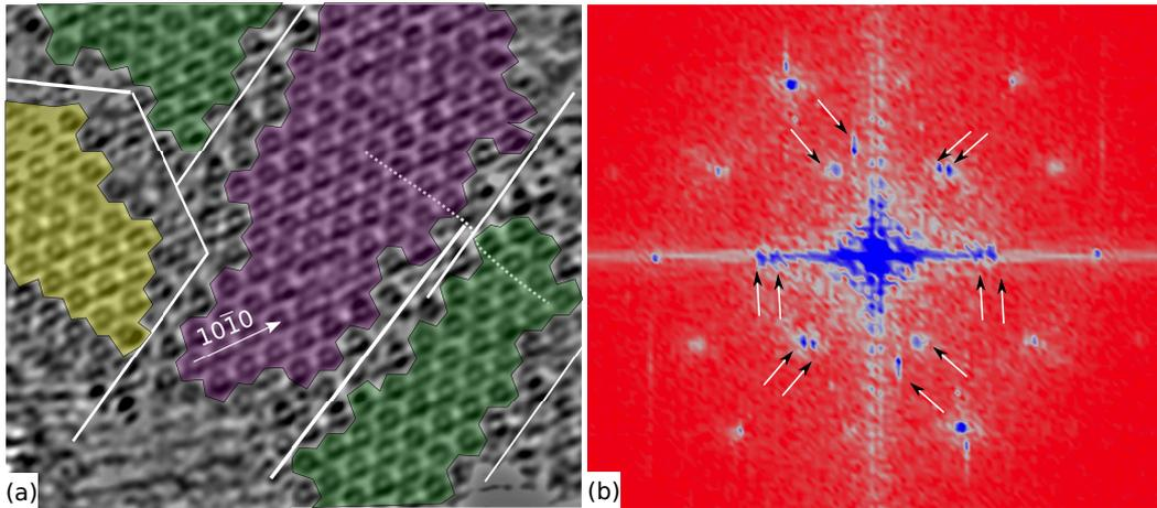
Figure 3.8: (a) Large scale STM image ( $9.5 \text{ nm} \times 8.5 \text{ nm}$ ) taken at  $0.9 \text{ V}$  tunnel bias and  $2 \text{ nA}$  tunnelling current. The anti phase domains of monolayer silicon oxide are highlighted in green, yellow and purple. The white lines mark the anti phase domain boundaries' orientation. (b) FFT of the STM image in (a). The splitting in the spots is demarcated by the white arrows with black pointers.
