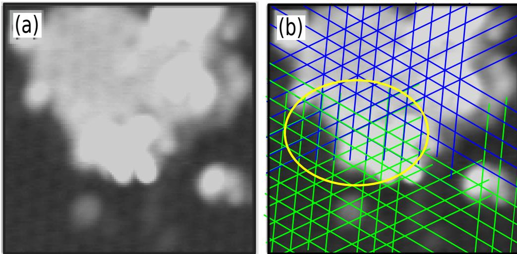
Figure 3.6: (a) STM micrograph of 30 % covering monolayer silicon oxide reported in the PhD thesis of L. Liechtenstein. The bright region is the monolayer silicon oxide surrounded by  $(2 \times 2) - 3O$  reconstructed Ru(0001) surface. Lines drawn in the oxygen lattice (green) marking the oxygen atoms or hcp-sites along with the centre of the hexagons (shown by blue lines). Adapted from [62].
