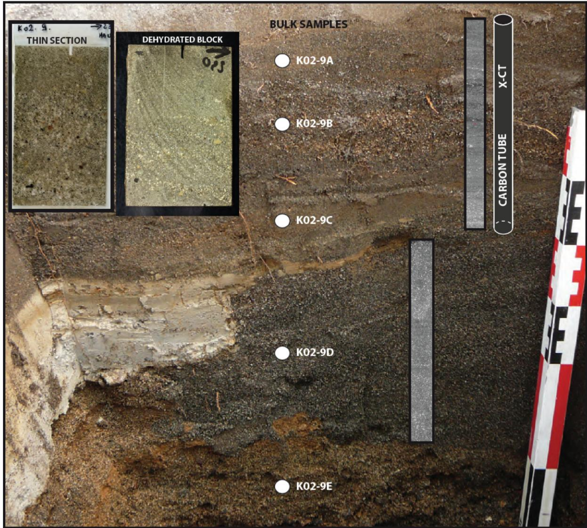
Fig. 3 – Example of sampling at site K02-9 (eastern shore of the lake). Bulk sampling of the 1996 tsunami deposit (K02-9A to K02-9D) and pre-tsunami sediments (K02-9E). The tsunami deposit is also sampled using carbon tubes (cores for X-ray tomography) and plastic boxes (for thin sections). Note the 20 cm-large rip-up clast of white ash at the base of the tsunami deposit.
