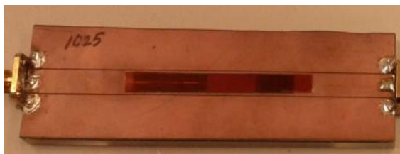
Figure II.23: La structure SIR recouverte de Kapton
