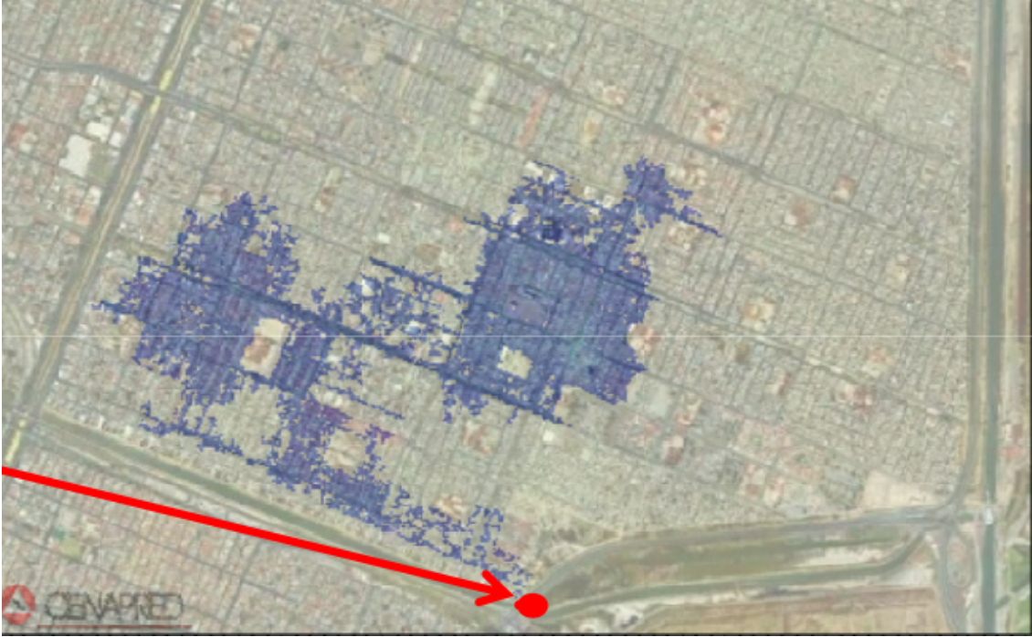
Figure 5.29 Northern flooded area where the Remedios channel enters the reservoir at the East of the airport, with point of hypothetical channel failure. [CONAGUA, 2011]
