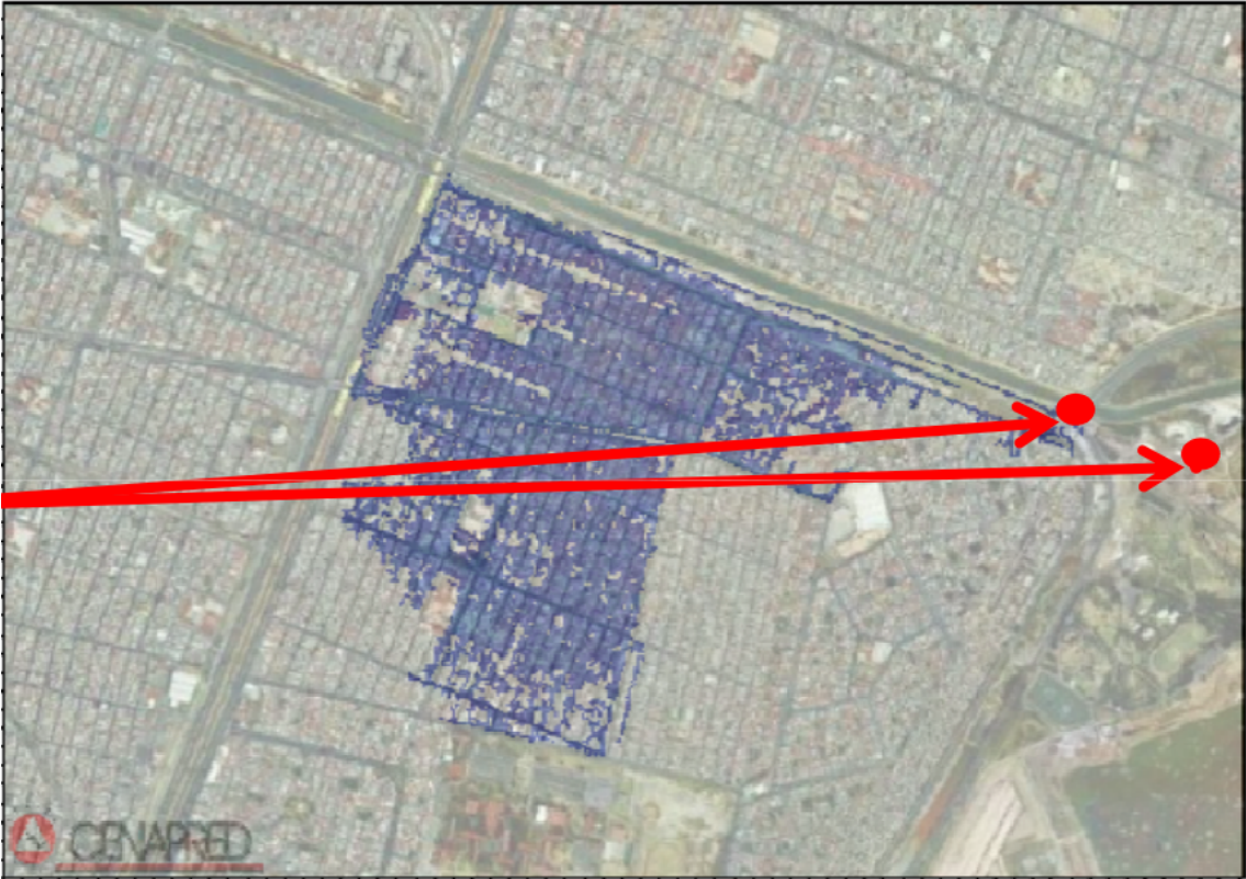
Figure 5.28 Southern flooded area where the Remedios channel enters the reservoir at the East of the airport, with points of hypothetical channel failure. [CONAGUA, 2011]
