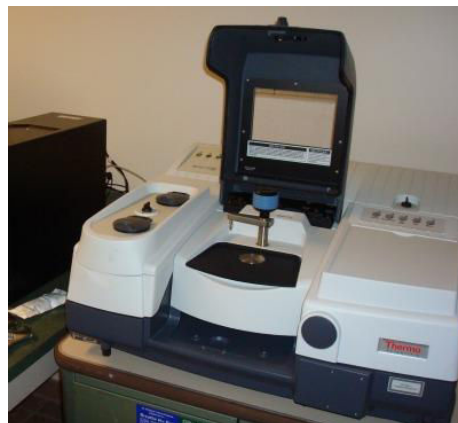
Fig. 5: a) ATR- Infrared Imaging Microscope (Nicolet iN10 MX), b) ATR-FTIR (Thermo-Nicolet)
