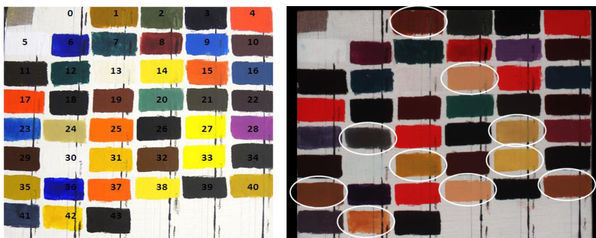
Fig. 67: Visible image (left panel) and "false" RGB image (right panel) of the pictorial layers spread on the lead white preparation. The "false" RGB image was obtained combined the images captured at 700, 650 and 500. The pictorial layers circled correspond to Raw Sienna Earth in position 1, Naples Yellow 14, Litharge 24, Zinc Yellow 27, Orpiment 31, Cadmium Yellow 33, Mars Yellow in position 35, Lead-Tin Yellow 38, Yellow Ochre in position 40 and Stil de Grain in 42.
