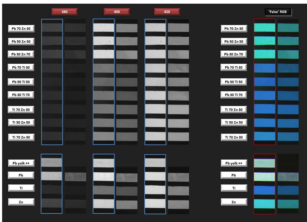
Fig. 150: Multispectral images at 380 nm, 400 nm and 420 nm of the white mixtures (left panel) and “false” RGB combination of the same images. The yolk samples are framed in blue in the multispectral images and in red in the “false” RGB image.
