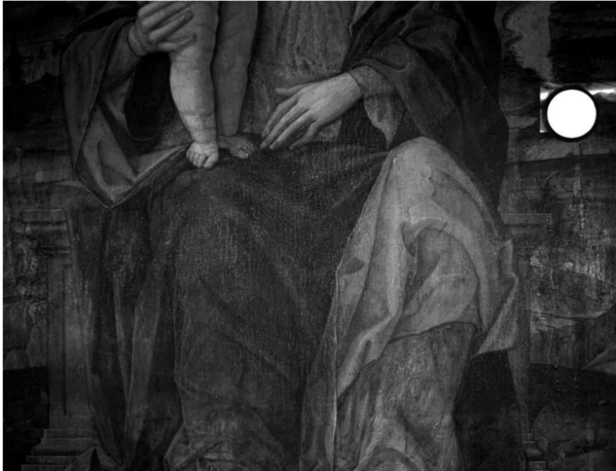
Fig. 15: Reflectance image of a painting with the reflectance standard
