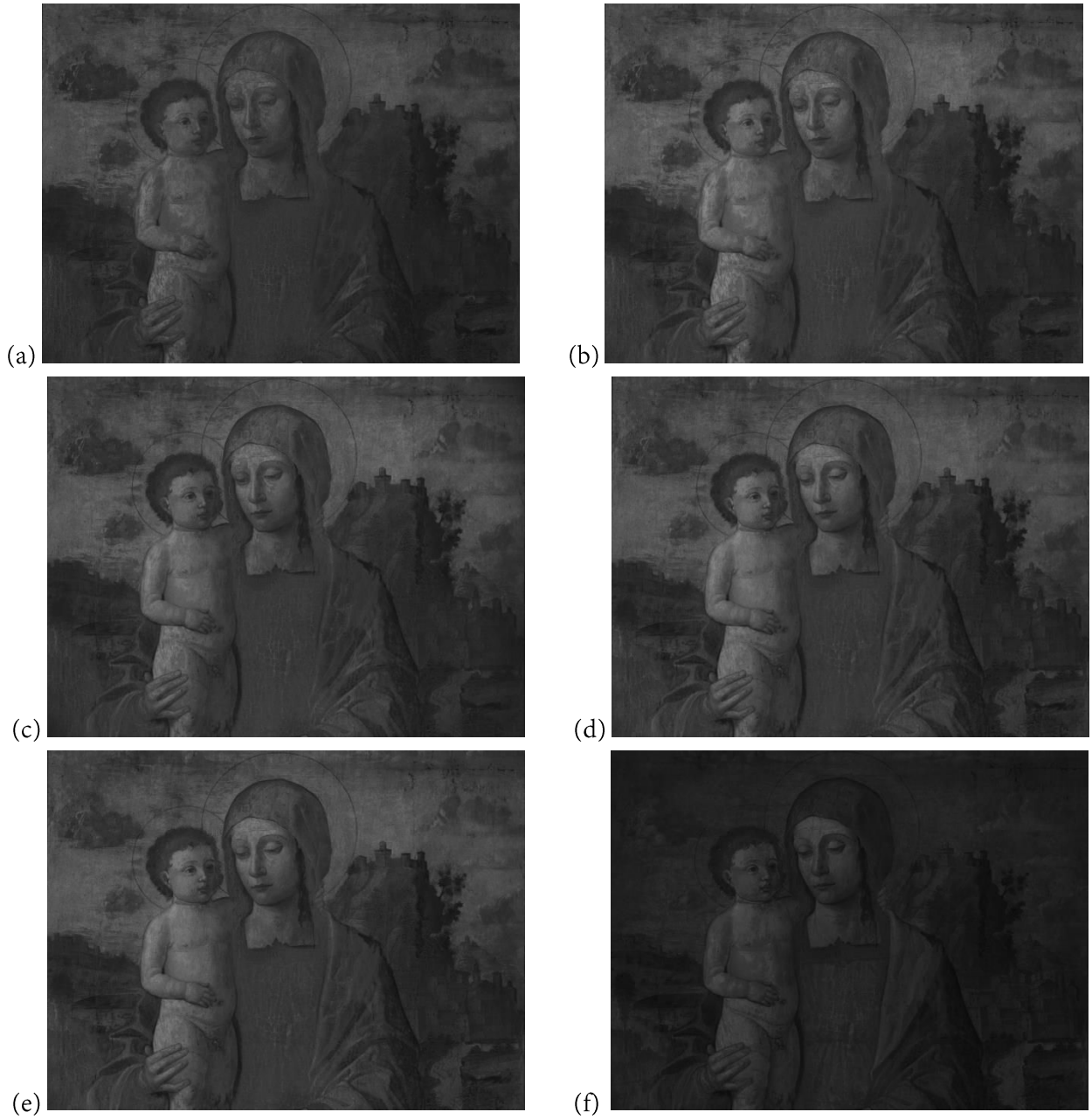
Fig. 218: Multispectral UV-fluorescence images at 450 nm (a), 470 nm (b), 500 nm (c), 532 nm (d), 550 nm (e) and 600 nm (f)
