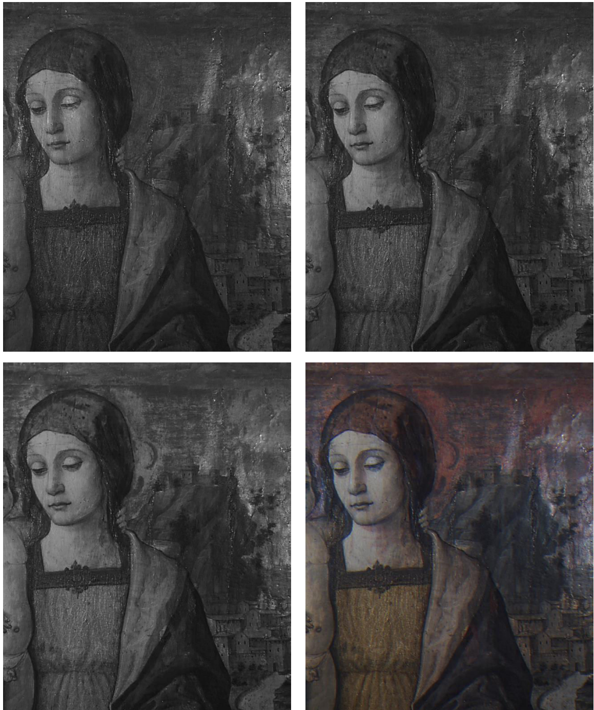
Fig. 228: Multispectral reflectance images at 600 nm (top left panel), 650 nm (top right panel) and 700 nm (bottom left panel) and “false” RGB reconstruction by using the above-mentioned images in the same order.
