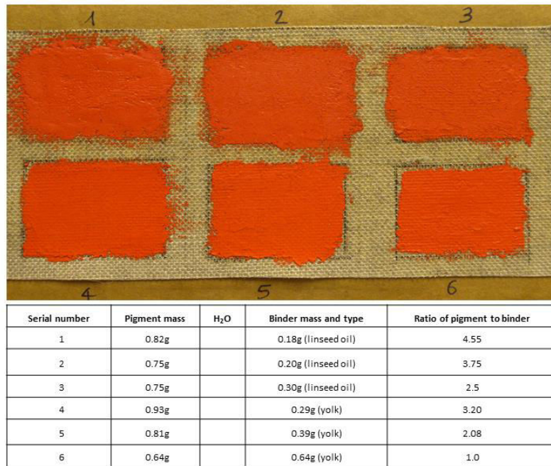
Fig. 91: Samples of Minium mixed with linseed oil or egg yolk.
