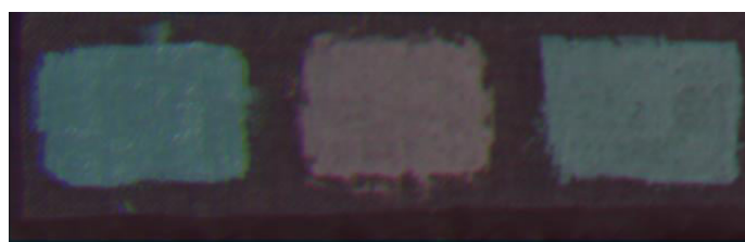
Fig. 135: From left to right: 'False' RGB combination of the multispectral reflectance images at 380 nm, 400 nm and 410 nm of the Zinc White with Hematite, Lead White with Hematite and the mixtures of Lead White, Zinc White and Hematite samples.
