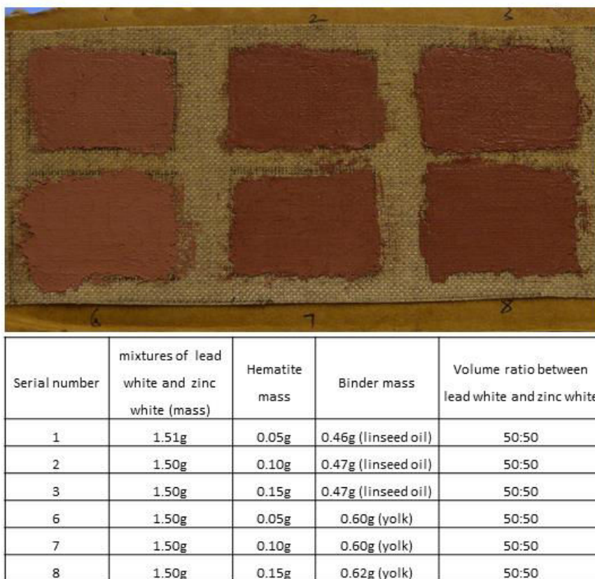
Fig. 100: Samples obtained mixing Lead White, Zinc White and Hematite with linseed oil or egg yolk.
