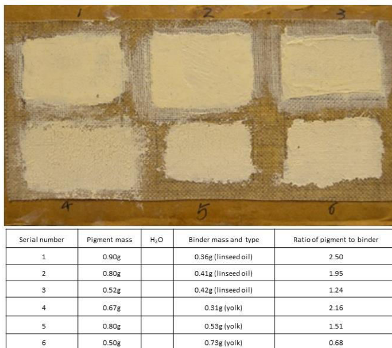
Fig. 95: Samples of Zinc White mixed with linseed oil or egg yolk.
