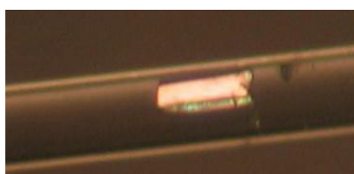
Figure 3.7: Picture of a single crystal of [Yb 2 (cda) 2 (ox)(H 2 O) 7 , 6H 2 O] ∞ in a glass capillary. Dimension: 0.14 x 0.04 x 0.05 cm 3 .
