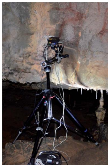
Fig. 3 Portable XRF apparatus implemented in La Garma Cave.
