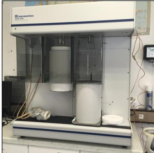
Figure 2-5 MICROMERITICS ASAP 2020
