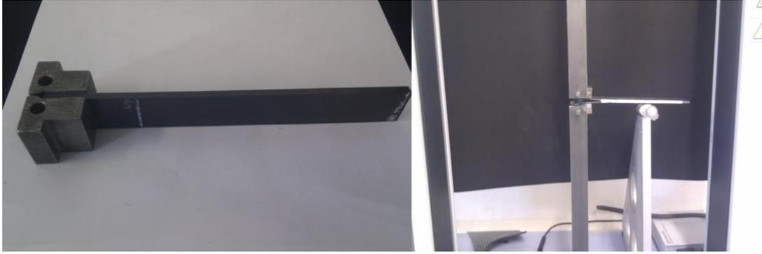
Figure III. 4. A picture of DCB specimen and test
