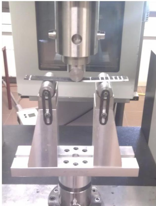
Figure III. 6. A picture of ENF test
