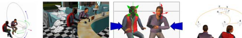
Figure 2.9 – Camera placement using the Toric Space allows quick calculation of framing specifications, and constructing long tracking sequences from keyframes [LC15].
