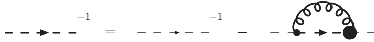
Figure I.2: Diagrammatic representation of the DSE for the ghost propagator Eq. (I.3.9). Dashed lines represent ghost propagators and wiggly lines gluon propagators. Bold lines and dots are full propagators and full vertices respectively, while normal ones are bare quantities. Original figure taken from [126].
