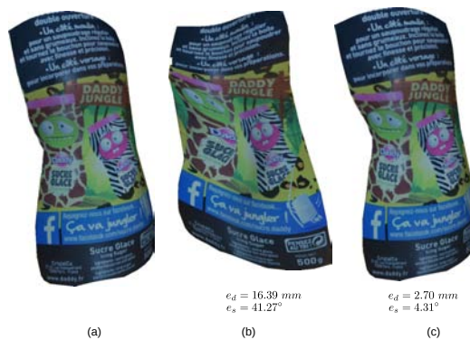
Figure II: Results: (a) ground truth (b) typell -P reconstruction with standard registration (c) typell -P reconstruction with robust registration.
