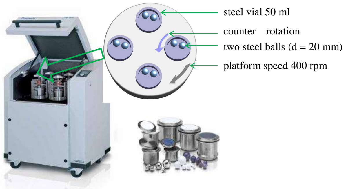
Figure 2-2 Retsch PM 400, vials and balls and present planetary mill setup
