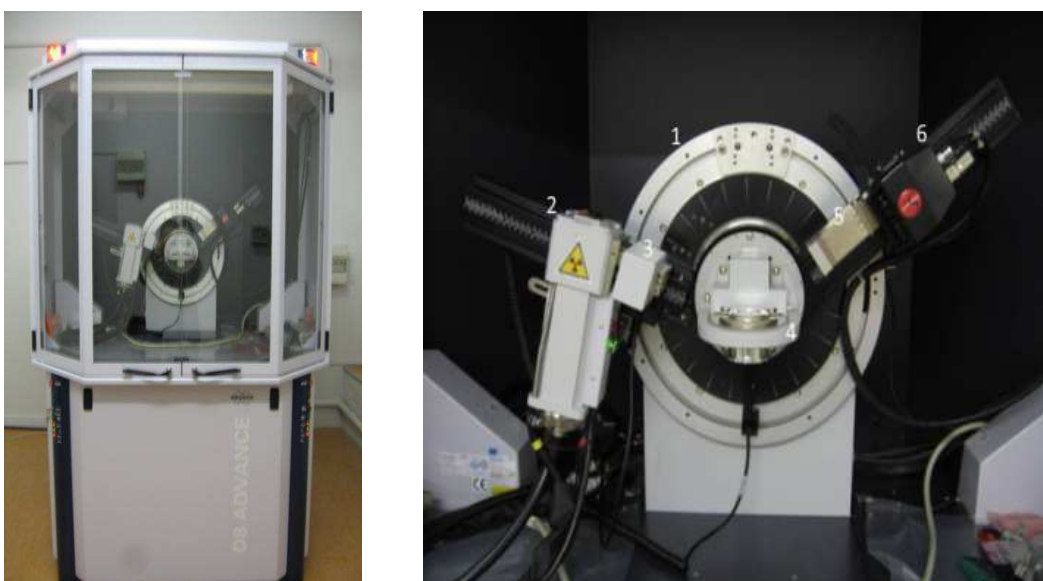
Figure 2-4 Bruker D8 Advance X-ray diffractometer (left) and Bragg-Brentano geometry (right)
