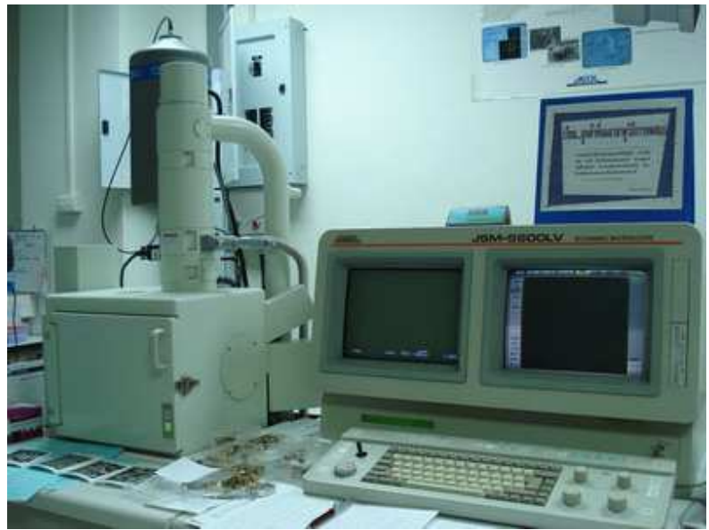
Figure 2-6 Scanning electron microscope scheme (left) and machine (JSM-5800LV) (right)
