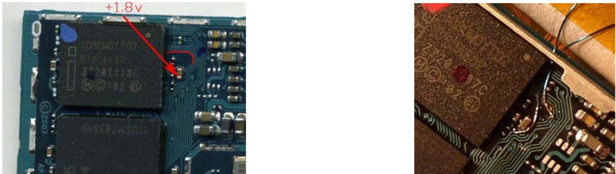
Figure 6.3: On the left, test points (red path and arrow) near the baseband processor where thin wires had to be soldered to pull the capacitor up (as depicted by the picture on the right), so the chip is tricked and will consider that the flash is erased. As a result, it will enter into a "recovery mode", where unsigned code can be downloaded without any verification. (images source: http://geohot.blogspot.fr/ )
