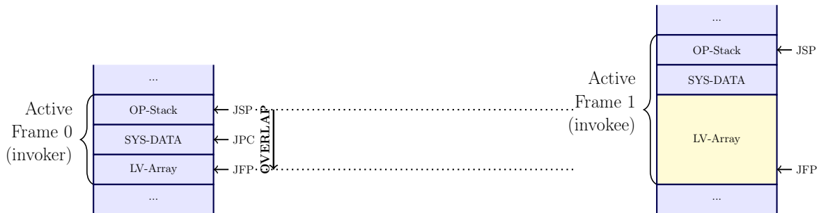
Figure 4.7: Frame bound expansion during method invocation
