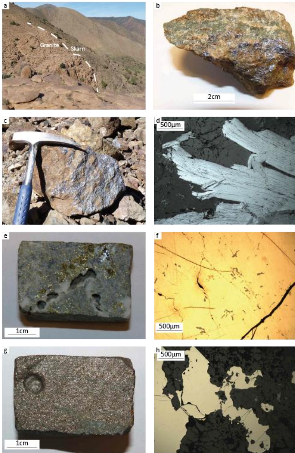
Figure IV-4: a) Granite and skarn contact in Azegour. b) Tizgui disseminated molybdenite in granatite. c) Coarse molybdenite from the Azegour mine. d) Azegour molybdenite. e) Chalcopyrite from Azegour mine. f) Chalcopyrite from Azegour mine. g) Pyrrhotite from Tizgui mine. h) Pyrrhotite from Tizgui mine.
