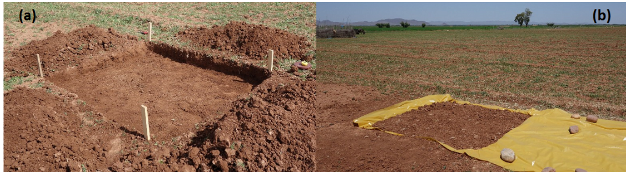
Figure 2. Illustration of the dry soil plot in the R3 perimeter. (a) The pit was dug at a 15-cm depth and (b) the soil plot was kept fully dry by covering it with a plastic sheeting in between experiments.
