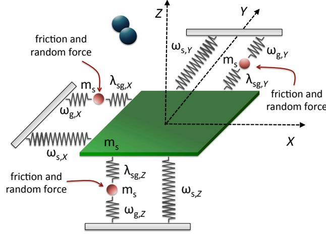
**Figure IV.1:** Schematic representation of the GLO model. The figure has been taken from Ref. [135].
