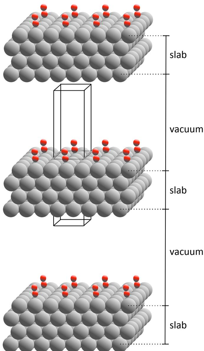
**Figure II.1:** Schematic representation of a  $3 \times 3$  supercell of a primitive surface unit cell with an diatomic molecule modelled by a slab of four layers which are separated by vacuum along the  $z$  direction. The supercell is indicated by the solid black lines.
