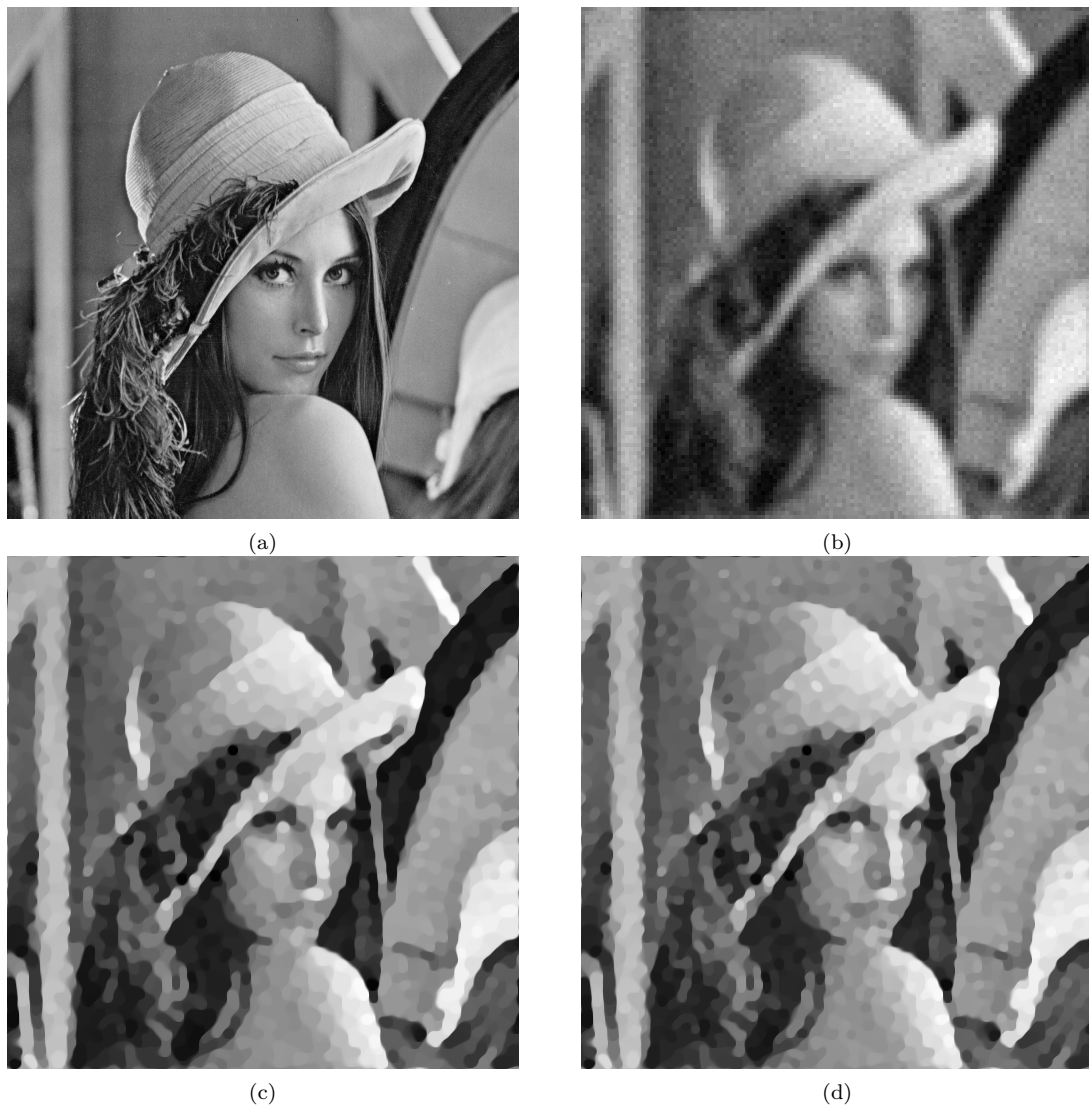
Figure 4.8: (a). Ground truth - Lena image; (b). Low resolution blurred and noisy image ( p = 4, \sigma_{blur} = 4.85, \sigma = 4.3 ); (c). Restored image with \mu_{DM} ; (d). Restored image with \mu_{UPRE} .
