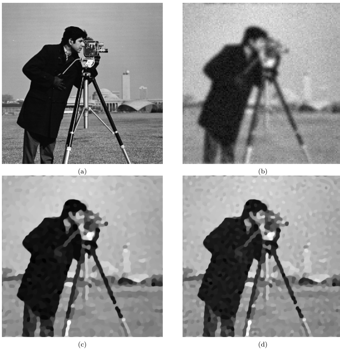
Figure 4.7: (a). Ground truth - Cameraman image; (b). Low resolution blurred and noisy image ( p = 4, \sigma_{blur} = 4.85, \sigma = 6 ); (c). Restored image with \mu_{DM} ; (d). Restored image with \mu_{UPRE} .
