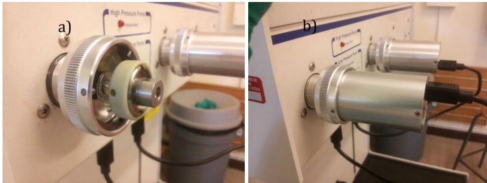
Figure 2-10 a) penetrometer placed into Low pressure chamber; b) Low Pressure Chamber on
