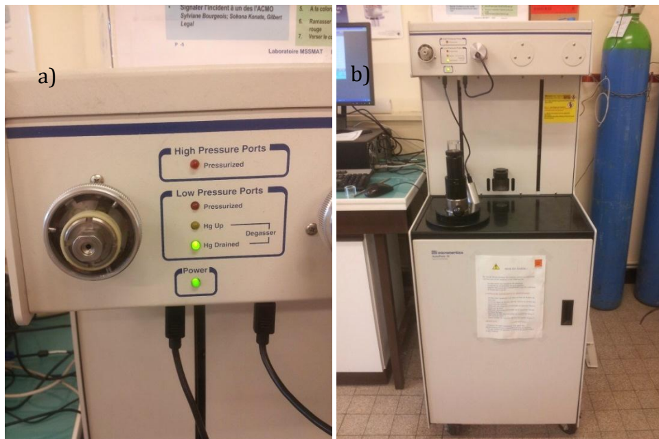
Figure 2-11 a) Low pressure analysis before beginning; b) AutoPore IV of Micromeritics (Model 9505/9500) Low Pressure and High Pressure Chambers
