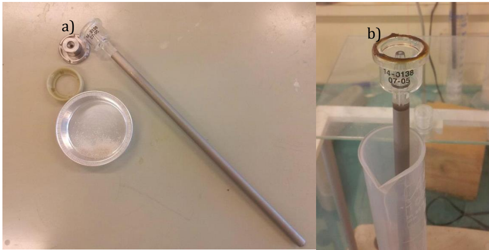
Figure 2-8 a) used penetrometer and Pumice sample; b) sample chamber
