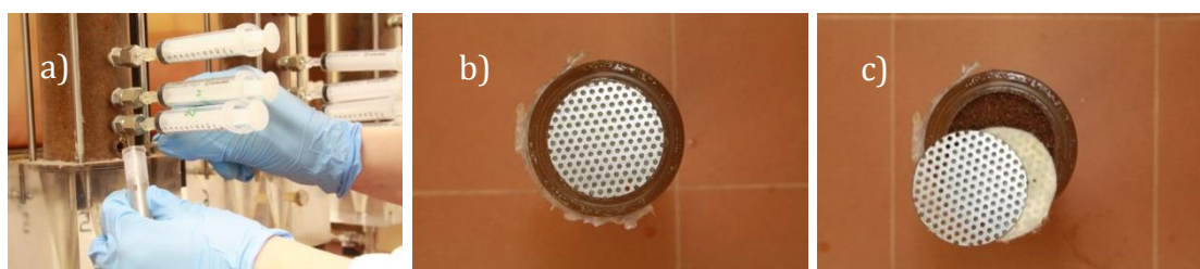
Figure 5-6 a) reactive material sampling, b) and c) two steps of column tests disassembling
