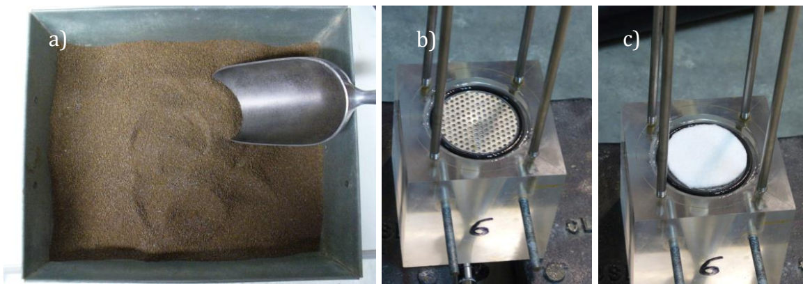
Figure 5-2 a) ZVI:Lapillus mixture; b) bottom of column with o-ring and inox grid; c) and with geotextile filter
